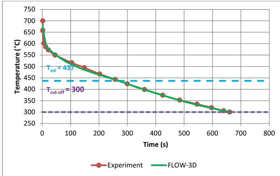
Figure 4: Evolution of temperature at the sprue-rod junction.
