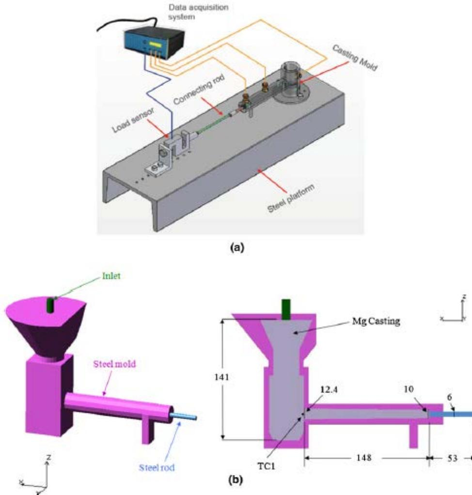
Figure 1: Experimental test setup: a) overall view and b) geometry of the casting and the mold as used in the simulations (all dimensions are in millimeters).
