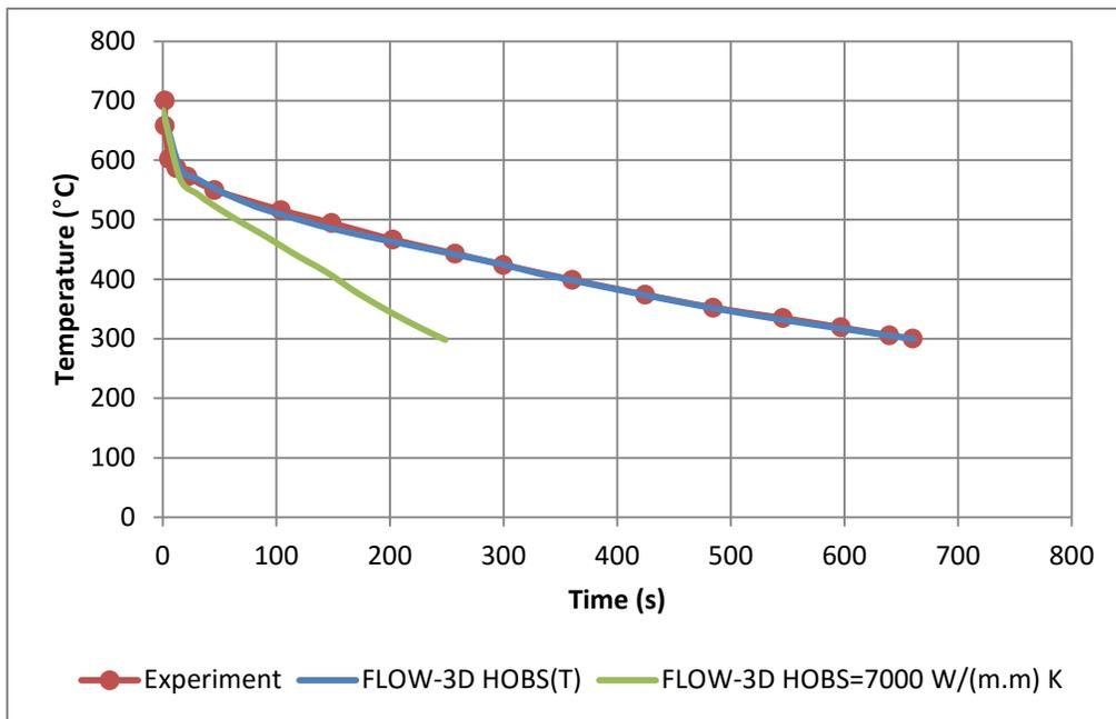
Figure 8: Evolution of temperature at the sprue-rod junction with constant and varying interfacial heat transfer coefficient, IHTC.
