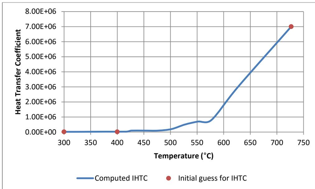
Figure 3: Computed interfacial heat transfer coefficient (IHTC) used for the *FLOW-3D* simulation.
