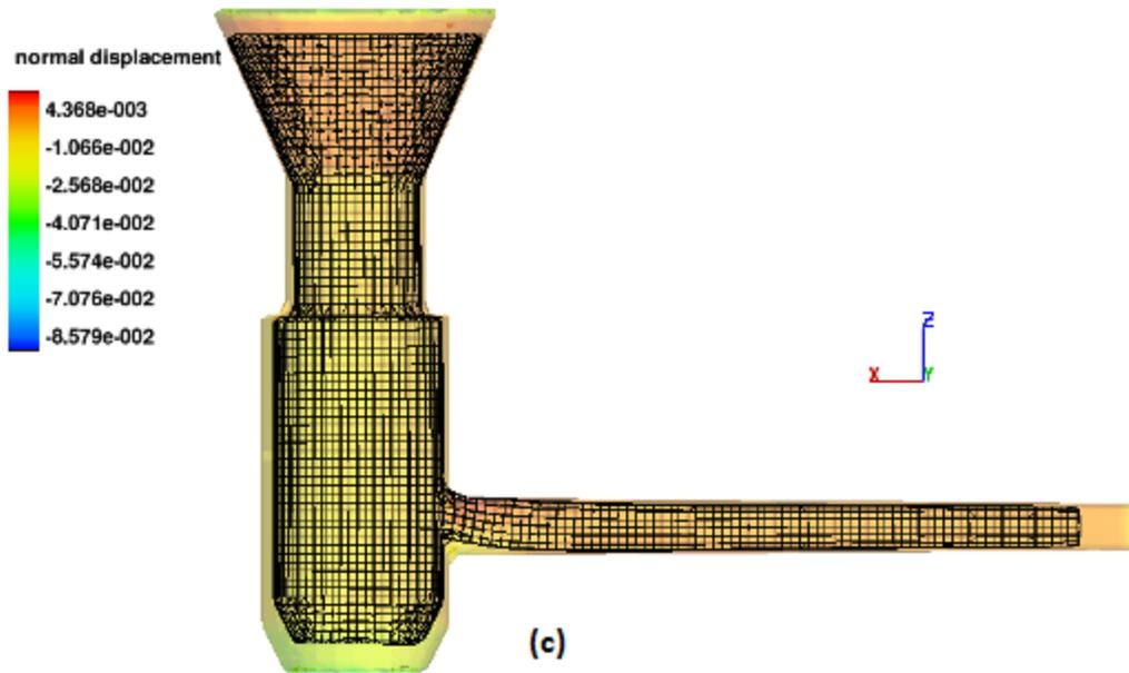
Figure 2: Predicted stress, strain and normal displacement at the end of solidification the Mg-9 wt. pct. Al,  $T_{\text{mold}} = 773\text{K}$  ( $500^{\circ}\text{C}$ ): a) x-direction stress, b) plastic effective strain, and c) normal displacement (magnified 20 times).
