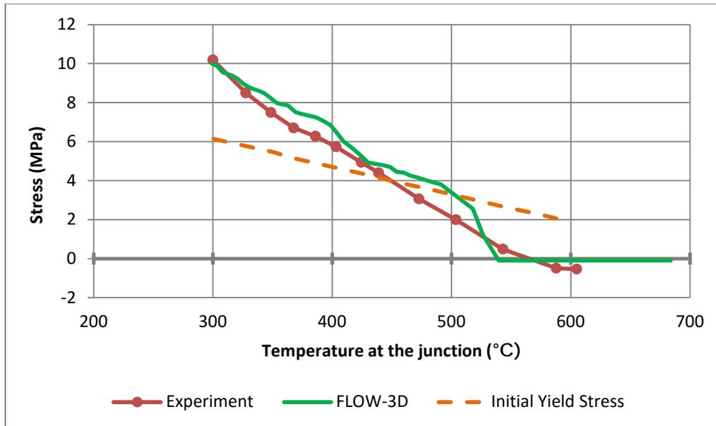
Figure 5: Average stress at the sprue-rod junction.
