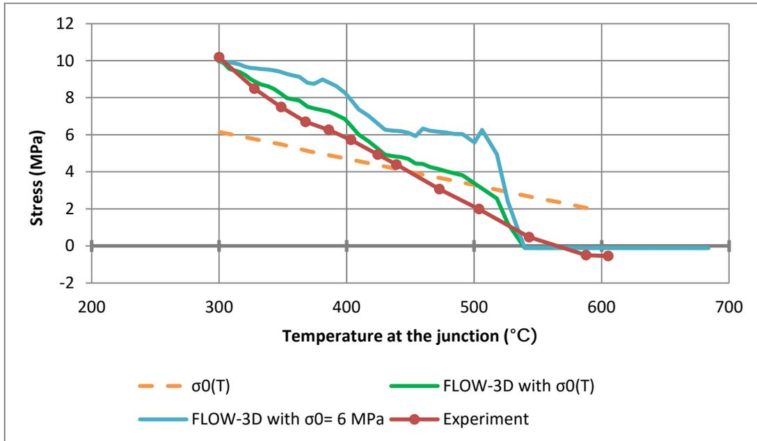
**Figure 6: Stress evolution at the sprue-rod junction with varying initial yield stress,  $\sigma_0$ .**
