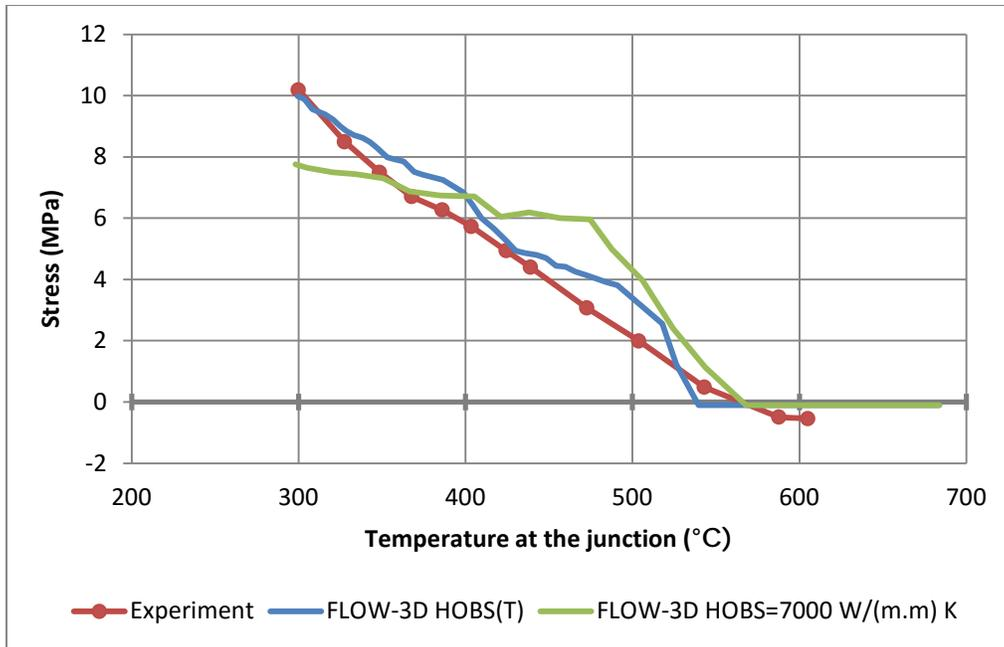
Figure 7: Stress evolution at the sprue-rod junction with varying interfacial heat transfer coefficient, IHTC.
