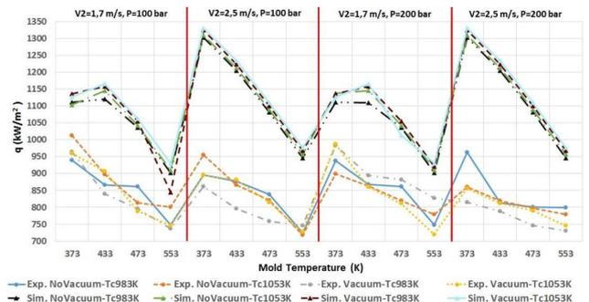
Fig. 6. Heat flux values calculated from experimental results and taken from simulations ( $\text{kW/m}^2$ ).
