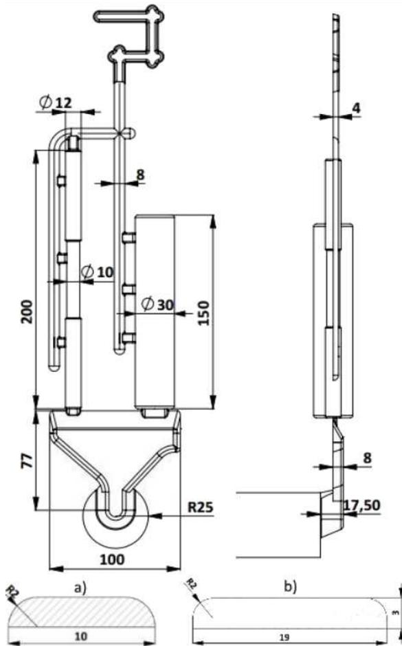
Fig. 1. The appearance of the parts, gating and vacuum channels used in experiments.
