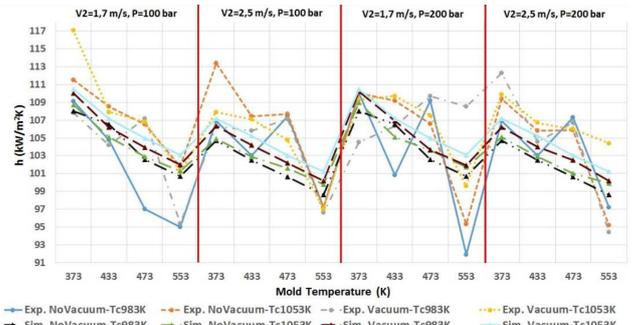
Fig. 5. IHTC results calculated from experimental results and taken from simulation ( $\text{kW/m}^2 \text{K}$ ).
