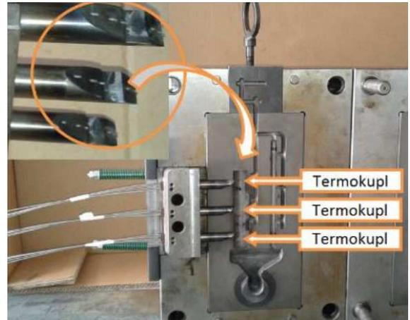
Fig. 2. Temperature measurement and thermocouple positioning.
