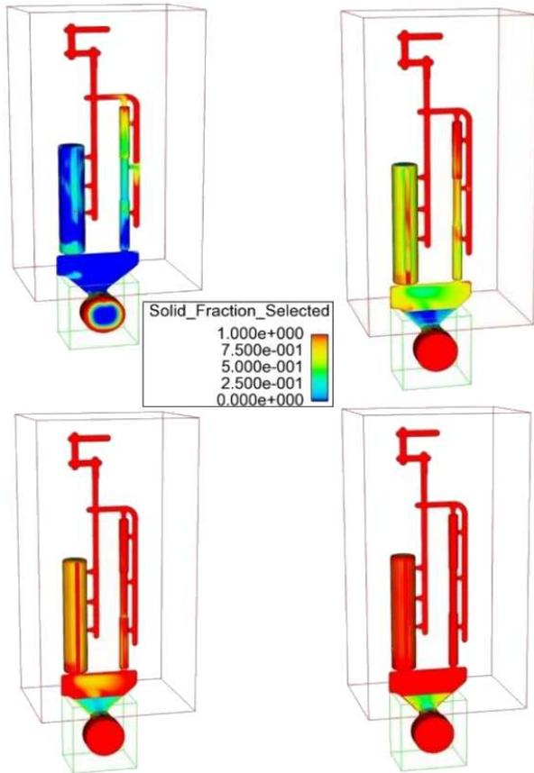
Fig. 4. The solidification simulation results from the simulation program.
