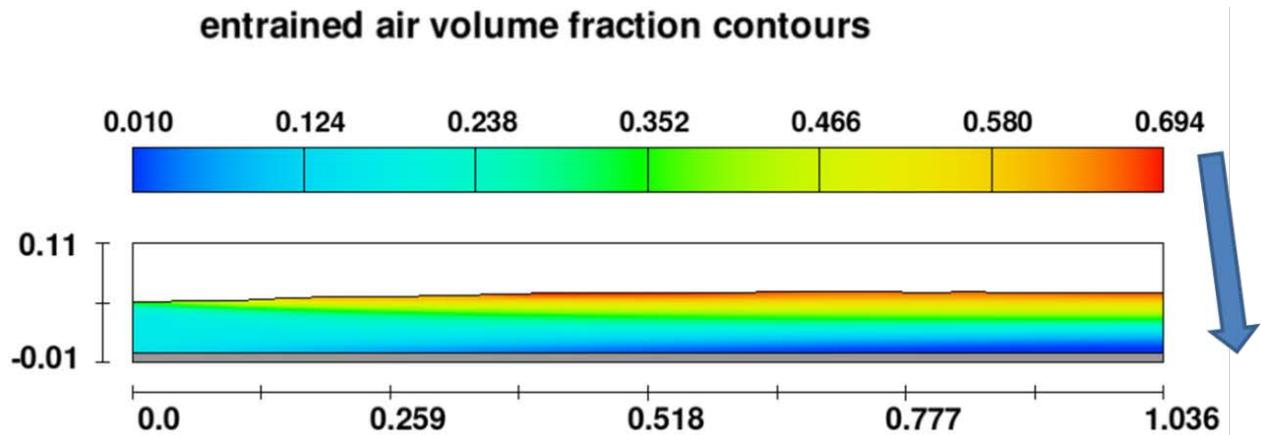
**Figure 6.** Air volume bulking up fluid in first meter down chute.
