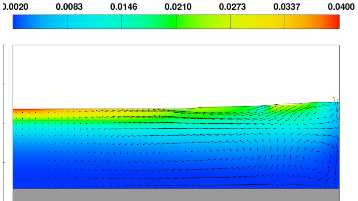
**Figure 7b.** Bubble diameter distribution at the end of chute (m).
