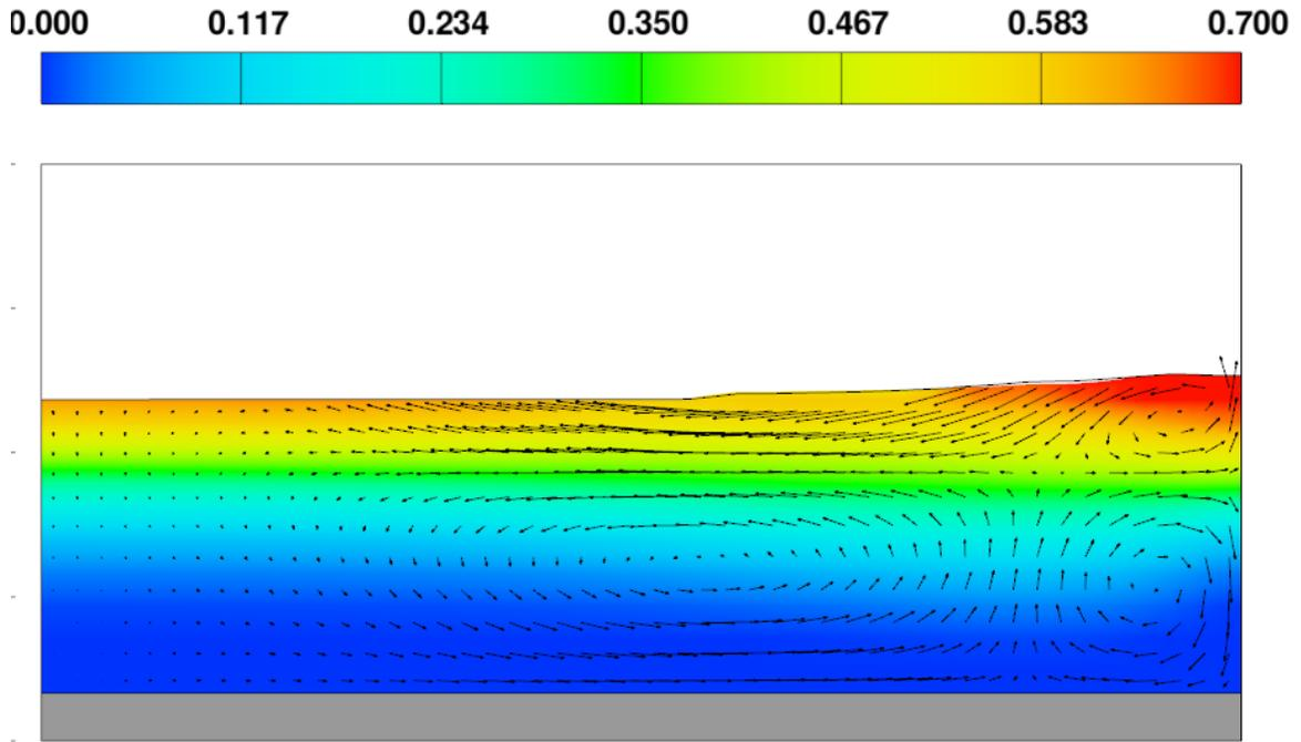
**Figure 7a.** Symmetric half of air concentration at end of chute.
