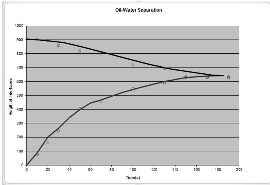
**Figure 1.** History of oil and water separation interfaces (oil at top, water at bottom). New model does not change droplet sizes because there are no mechanisms for coalescence or breakup. Solid lines are experimental values and circles are simulation results.
