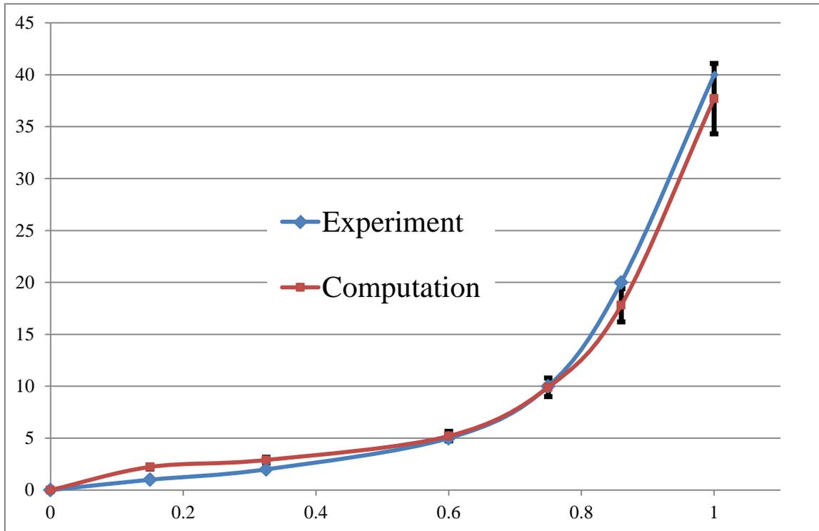
**Figure 8.** Computed bubble diameters from floor of chute to top of water in comparison with experimental data at the end of the chute. Errors bars on the computational results indicate variations with time since the solution is only quasi-steady.
