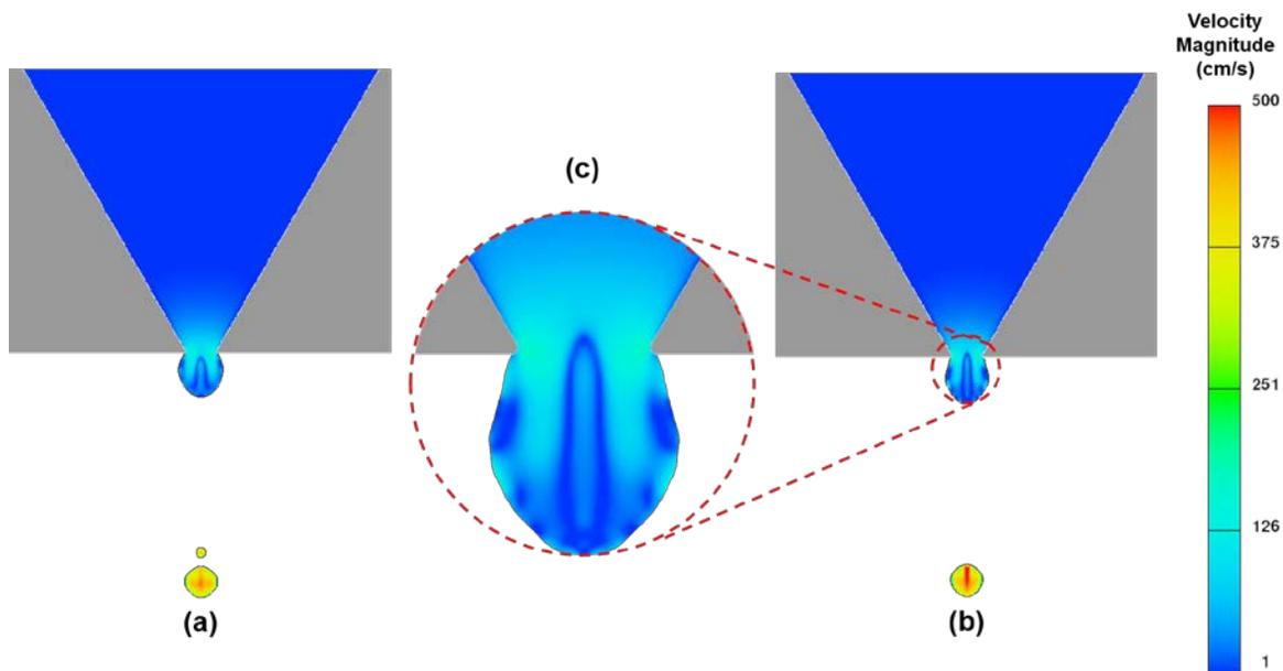
**Figure 3.** CFD analysis of droplet generation showing fluid velocity magnitude (cm/s): (a) droplet ejection in vacuum, (b) droplet ejection in atmospheric conditions, (c) inset showing fluid deformation after the applied pressure pulse and the geometrical details of the nozzle.
