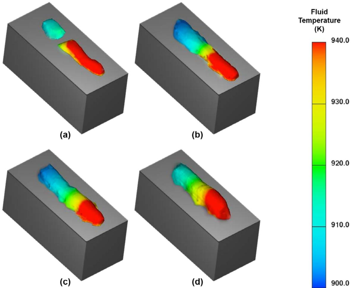
**Figure 4.** Parametric CFD analysis of the effects of ejected droplet ( $R=250\mu\text{m}$ ) separation distance (center to center) on the creation of a 4mm 3D printed line showing fluid temperature (K): (a) droplet spacing of  $650\mu\text{m}$ , (b) droplet spacing of  $500\mu\text{m}$ , (c) droplet spacing of  $300\mu\text{m}$ , (d) droplet spacing of  $200\mu\text{m}$ .
