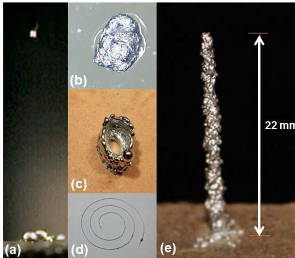
**Figure 5.** Droplet generation and droplet-media interactions: (a) jetted aluminum droplet in flight, (b) aluminum droplet solidified on a plastic substrate, (c) solidified printed ring structure, (d) spiral pattern of printed droplets after solidification, (e) printed pillar of coalesced aluminum droplets.
