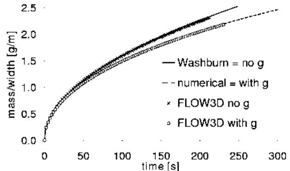
Figure 14: Diagram of fluid volume inside the screen versus time.
