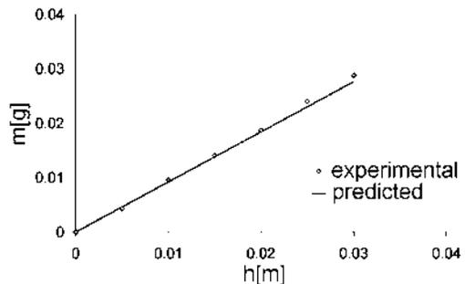
Figure 3: Graph of the liquid mass inside the wick plotted versus wicking height (HFE in 16 mm wide mesh)
