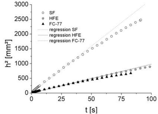
Figure 11: Height<sup>2</sup> over time with linear fitting (no error bars for graph clarity).
