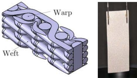
Figure 2: Drawing of the microstructure (left) and photography (right) of the Dutch-Twilled-Weave mesh (DTW)  $200 \times 1400$  (supplier: Spoerl).
