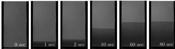
Figure 9: Wicking of the mesh using HFE for increasing time.
