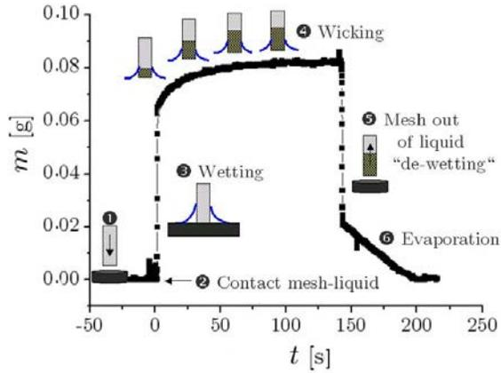
Figure 8: Description of the mass versus time curve (open test chamber). Imbibition of a mesh (50x16) by HFE.
