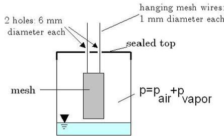
Figure 5: Sketch of the test chamber prior to wicking experiments.
