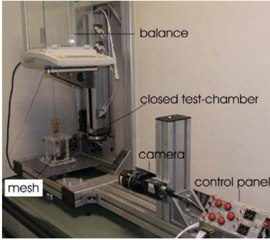
Figure 4: Photography of the wicking experimental setup.
