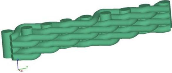
Figure 13: Digital representation of the screen showing its microscopic structure.
