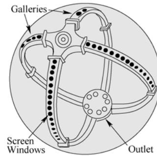
Figure 1: Propellant management device [5].
