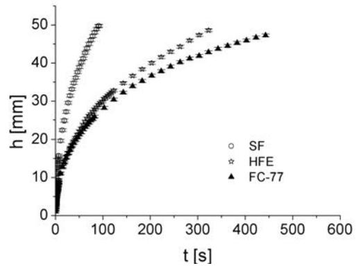
Figure 10: Wicking height raw data with error bars (standard deviation is  $\pm 5$  pixel).
