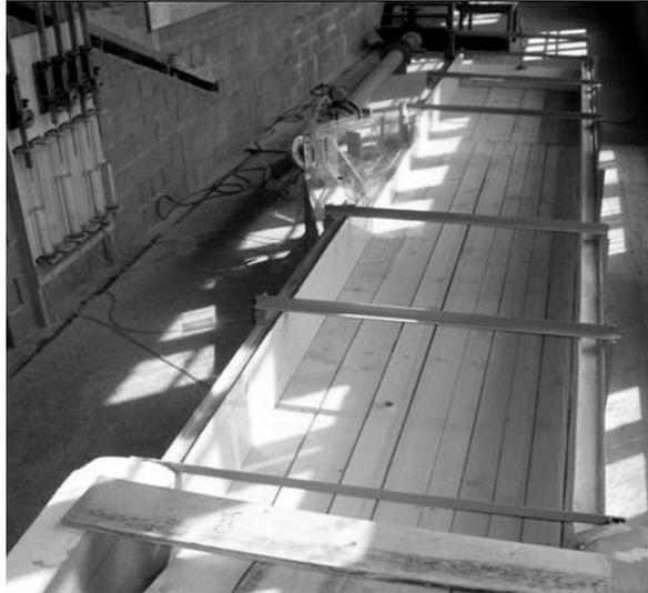
*Fig. 1. Hydraulic intake model in the scale 1:20.*
