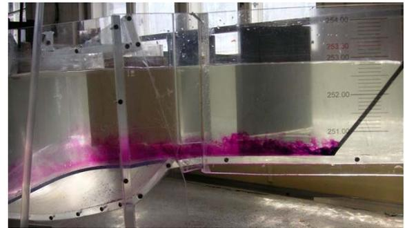
Fig. 5. Proposed form of the intake bottom
