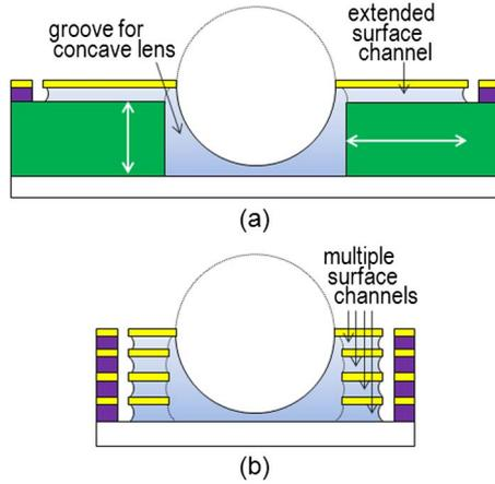
Fig. 6. (Color online) Schematic cross sections of the MEFL for enlarging the optical power by lowering the channel height; (a) a larger surface channel and (b) multiple surface channels.
