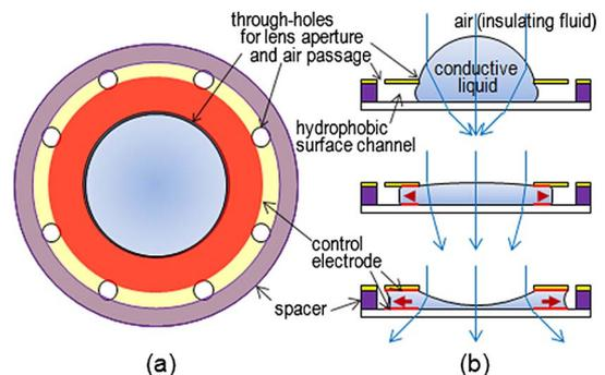
Fig. 1. (Color online) Schematic of the MEFL; (a) top and (b) cross-sectional views.
