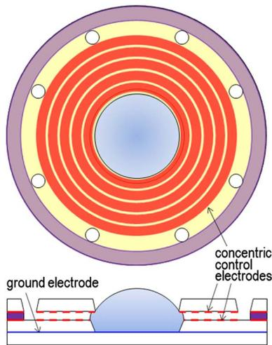
Fig. 2. (Color online) Schematic of the digital MEFL having concentric control electrodes.
