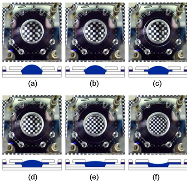
Fig. 3. (Color online) Experimental results of the fabricated MEFL and the schematic cross-sections; TCL radii of (a) 1.8 mm, (b) 2.0 mm, (c) 2.3 mm, (d) 2.6 mm, (e) 2.9 mm, and (f) 3.2 mm.
