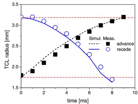
Fig. 4. (Color online) Experimental and simulation results of time-dependent TCL position in the MEFL.
