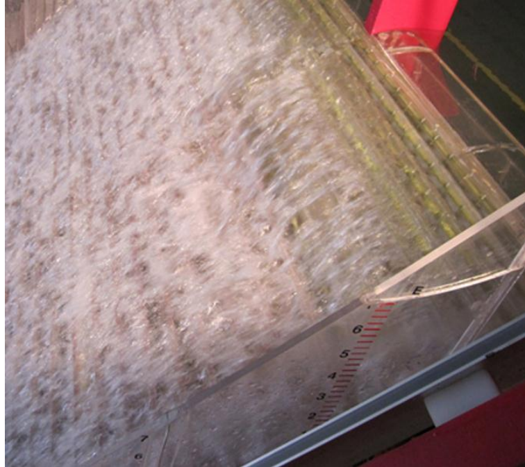
Figure 7. Regulated flow in the proposed design of physical model, passing low discharge
