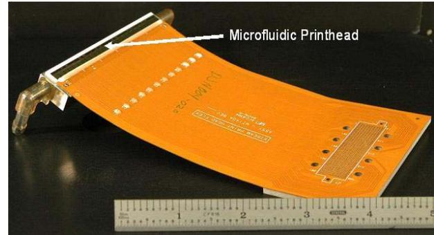
Figure 8: Fabricated microfluidic printhead.
