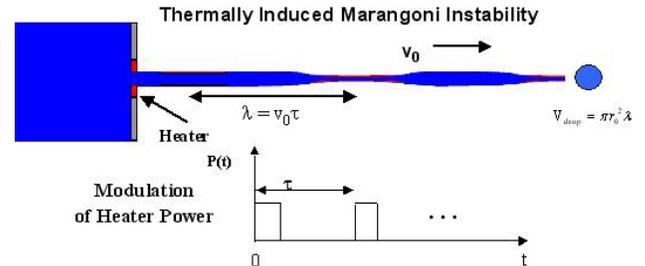
Figure 1: Illustration showing a single nozzle with an integrated heater at the orifice, and a thermal modulation pulse used to induce Marangoni instability and drop formation.
