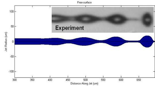
Figure 5. Slender jet analysis vs. experimental data.
