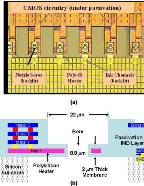
Figure 2: Inkjet printhead: (a) top surface of liner array of nozzles, (b) cross-section of nozzle/heater structure showing CMOS circuitry.
