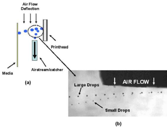
Figure 7: Continuous inkjet printing: (a) schematic showing drop size selective printing, (b) experimental picture showing airflow induced separation of large and small drops.
