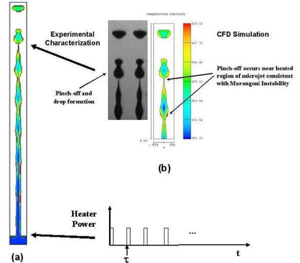
Figure 6. CFD simulation and comparison with experiment.
