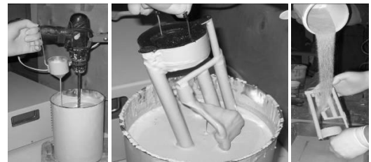
Fig. 18. Viscosity measurement with Ford cup. Making first layer of ceramic mould
