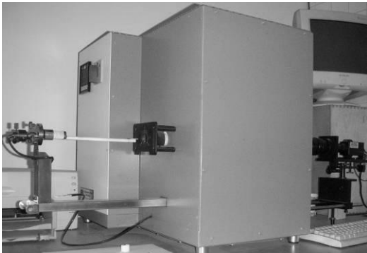
Fig.1. PR-25/1750 apparatus for the determination of characteristic temperatures
