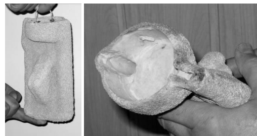
Fig. 20. Ceramic mould in layers. Mould after melting out of pattern material
