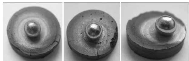
a) substrate – binder ZrO 2 +ZrO 2 , 1810°C, 2min; b) substrate – binder CeO 2 +ZrO 2 , 1800°C, 5min; c) substrate – binder Y 2 O 3 +ZrO 2 , 1800°C, 5min
