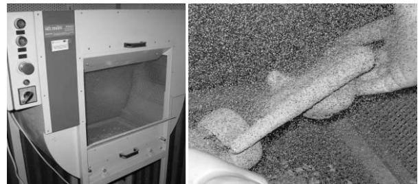
Fig. 19. Making subsequent layers of ceramic mould
