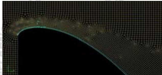
Fig. 4. Meshing and its distribution in the model of ogee spillway [21]
