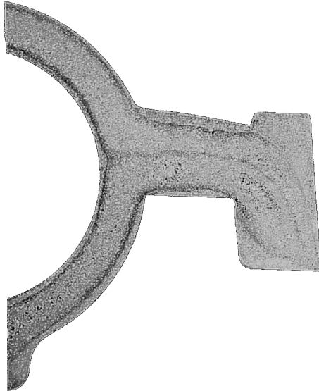
Fig. 10: Microstructure in the area of the inlet of the overflow
