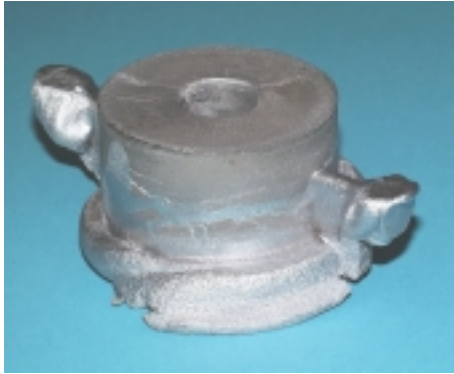
Fig. 7: Form filling of the elementary work piece. The punch stroke was equal to the simulation shown in Fig. 6
