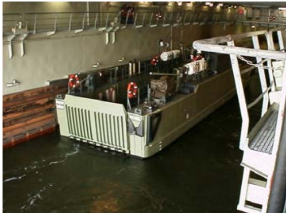
Figure 2, Single landing craft inside well deck of HNLMS Rotterdam
