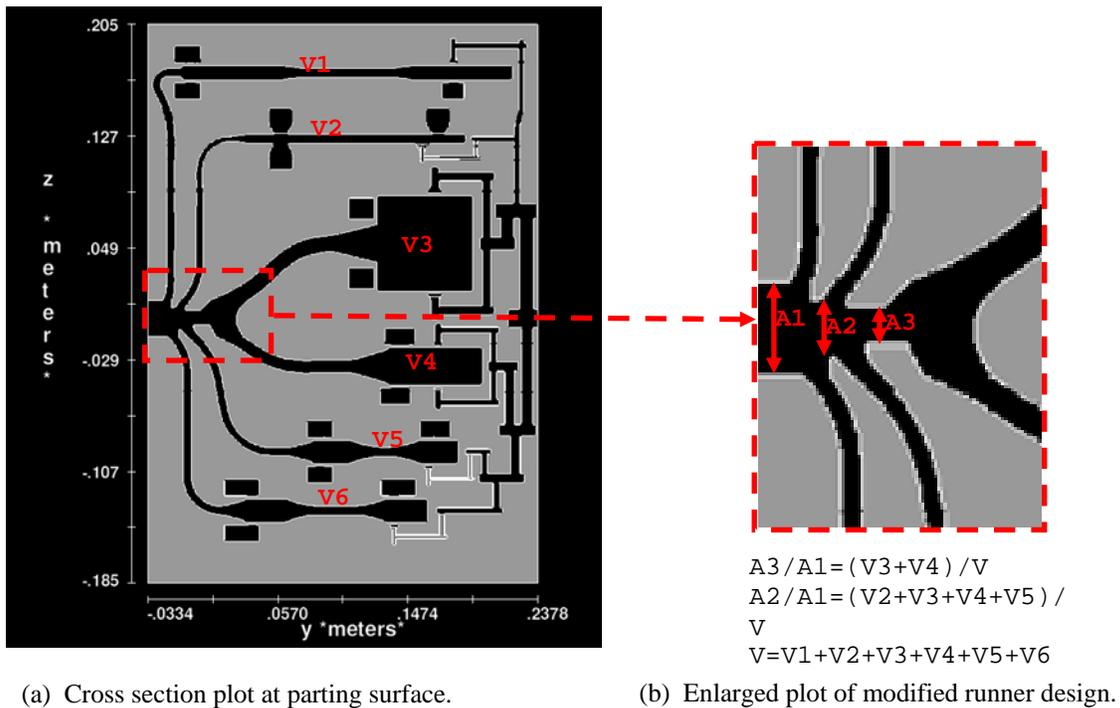
**Figure 4- Cross section at parting surface of ejector insert for modified runner design.**
