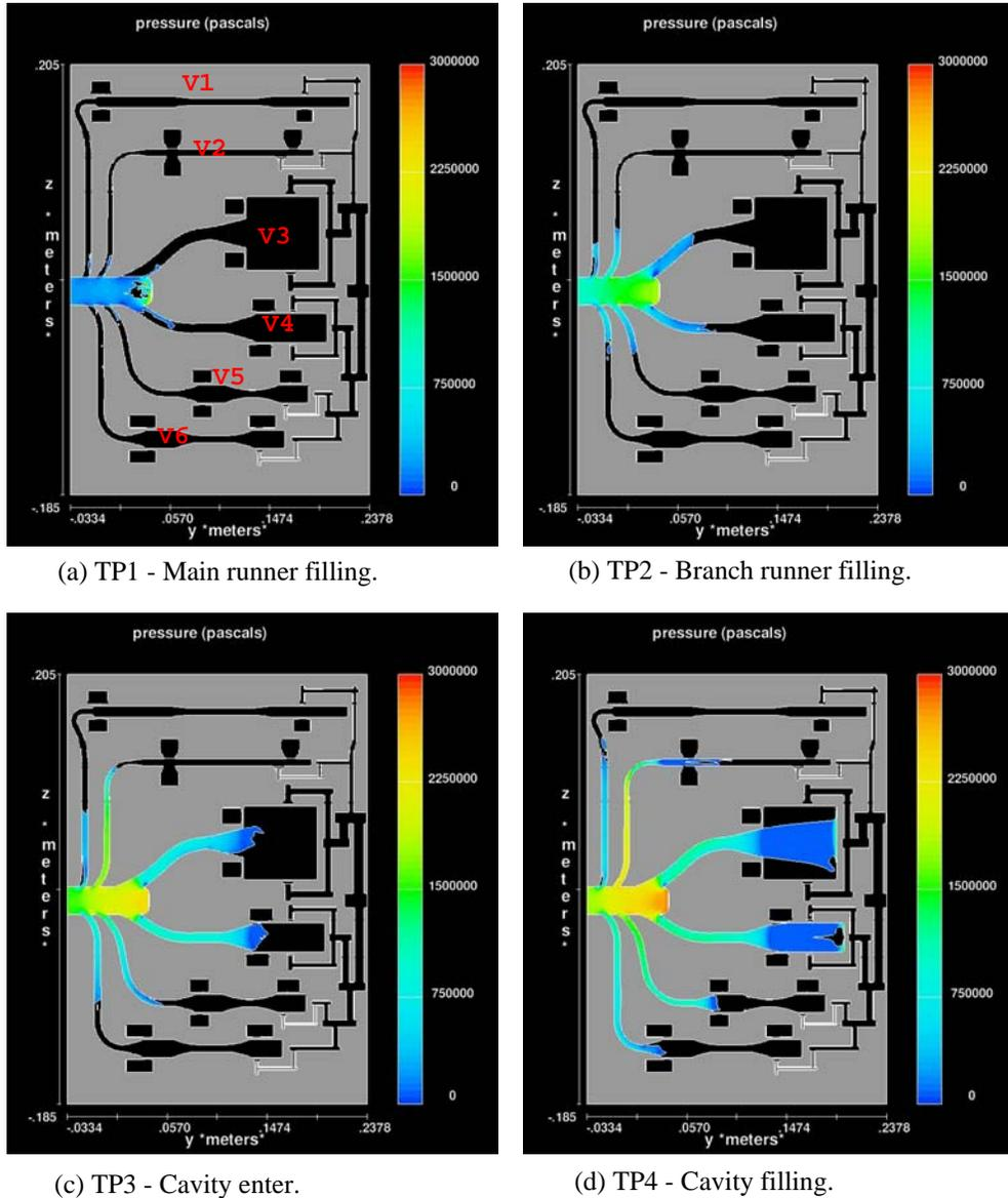
**Figure 3- Computed pressure contour along parting surface at different time point (TP) as metal filling the die cavities for original runner design.**
