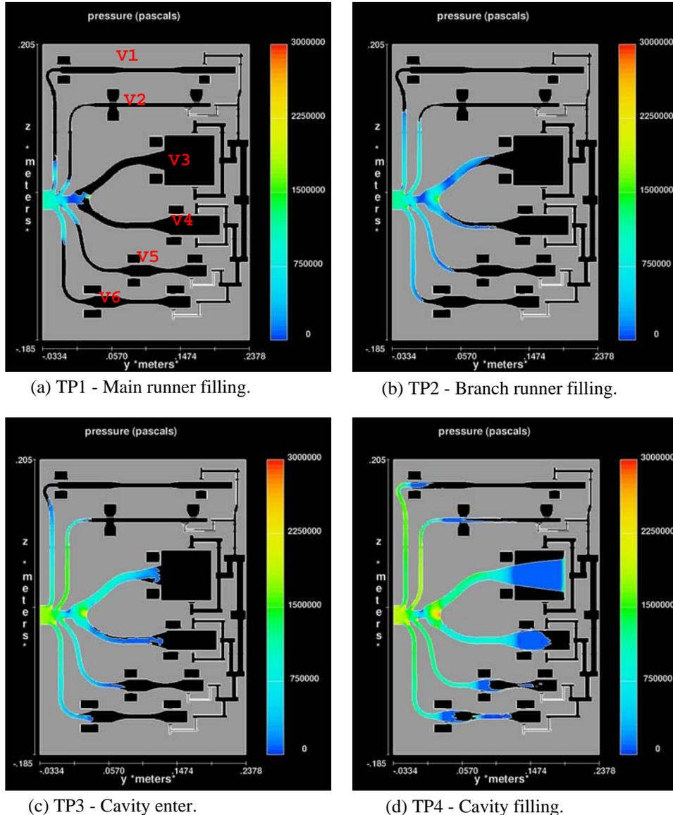
**Figure 5- Computed pressure contour along parting surface at different time point (TP) as metal filling the die cavities for modified runner design.**
