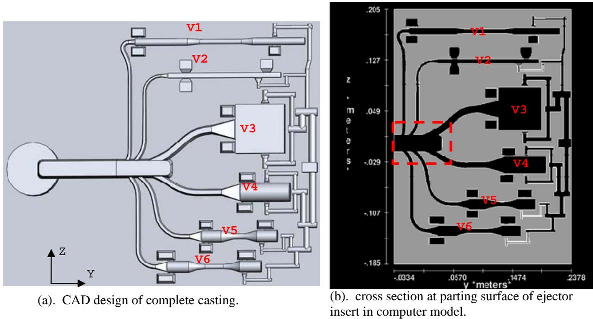
Figure 2- CAD design of complete casting (a) and cross section at parting surface of ejector insert in computer model (b) for original runner design.
