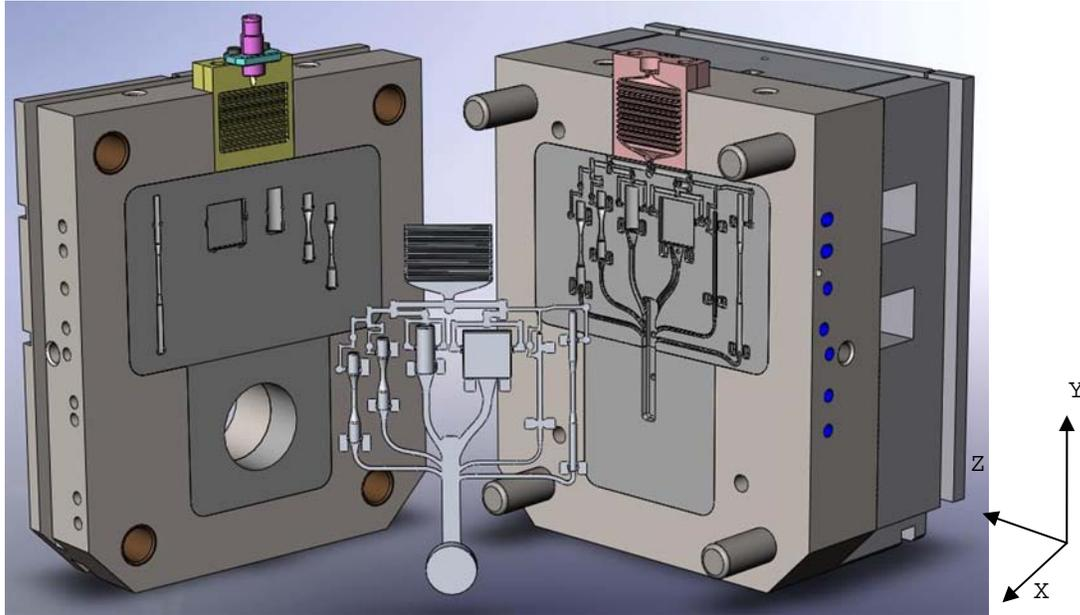
Figure 1- CAD design of die assembly and casting part. Gravity direction is along the negative y direction. Shot sleeve and plunger are aligned along the x direction.
