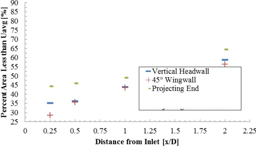
Figure 3. Percentage of the cross sectional flow area with streamwise velocity less than  $U_{avg}$ .
