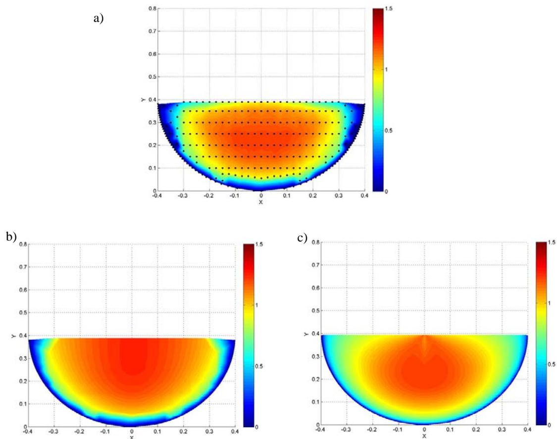
Figure 5. Normalized streamwise isovels for a) measured data, b) Flow3D predictions, c) Clark and Kehler (2011) predictions.
