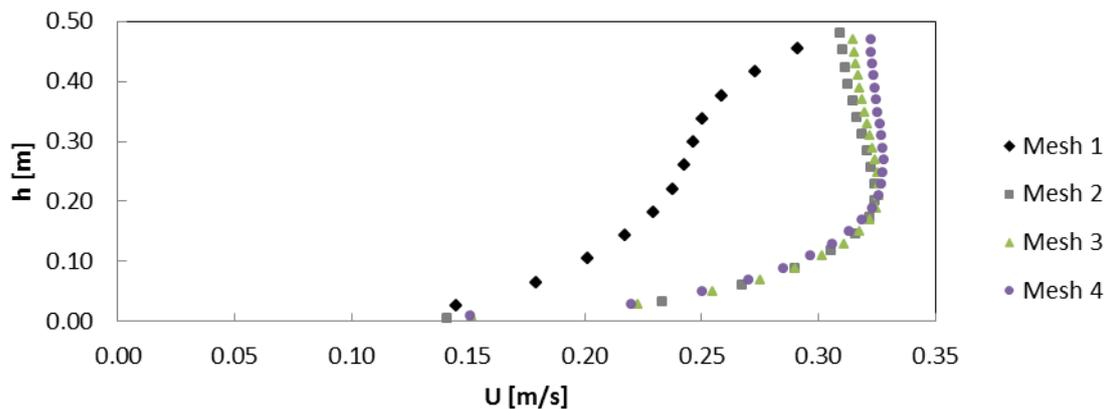
Figure 4. Centreline streamwise velocity profiles for several Flow3D runs using different meshes.
