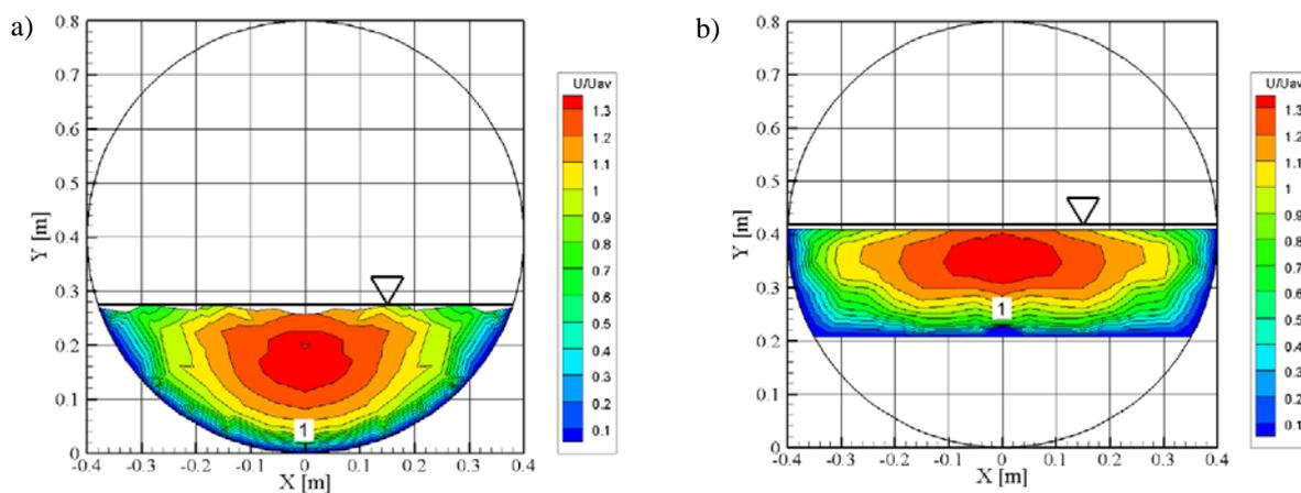
Figure 1. Normalized isovels for a) non-embedded fully developed flow, and b) fully developed flow with 30% gravel embedment.
