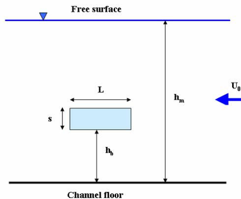
Fig. 3: Experimental Configuration
