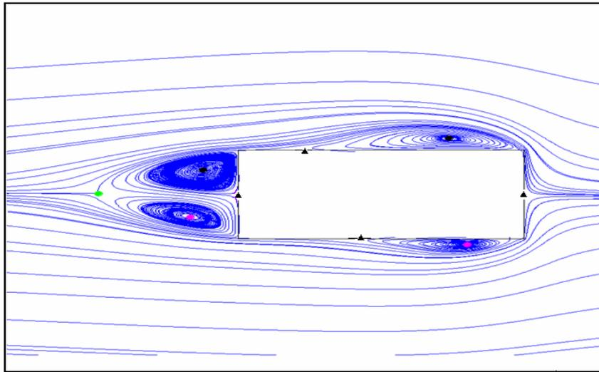
Fig.5: Mean flow structures ( $h_b/s=2.33$ ,  $h^*=5$ ); ●, anticlockwise vortex; ■, clockwise vortex; ▲, saddle points. (Present work)
