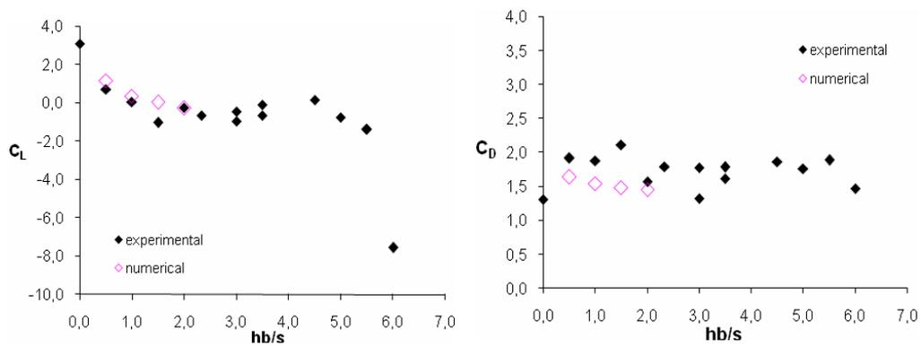
Fig. 15: Comparison of mean hydrodynamic coefficients. (experimental [1]; numerical [present work])
