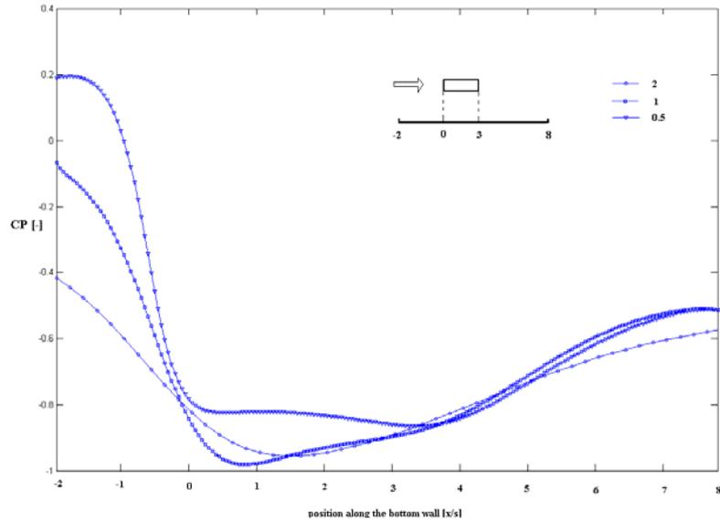
Fig. 14: Pressure distribution along the bottom wall.
