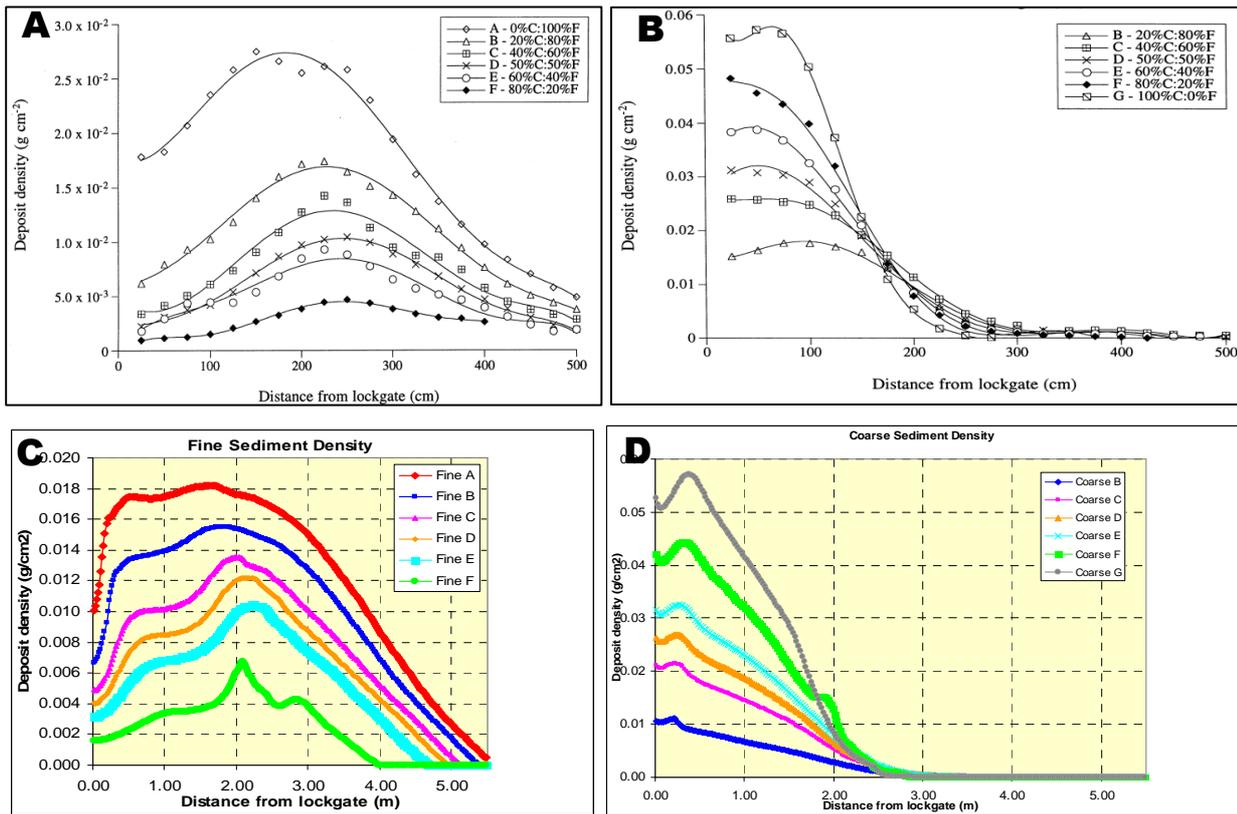
**Fig. 2.** (A & B) Laboratory measurements of ‘deposit density’ along the flume floor, for flows with different percentages of coarse (C) and fine particles (F). (C & D) The corresponding results from numerical simulated flows.
