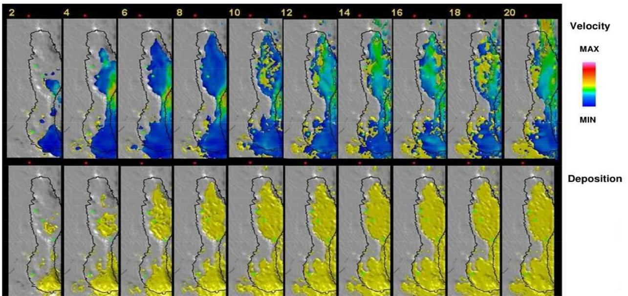
**Fig. 3.** Plan-view snapshots of the velocity field of successive flows (top) and the corresponding pattern of sand accumulation in the Ormen Lange sub-basin.
