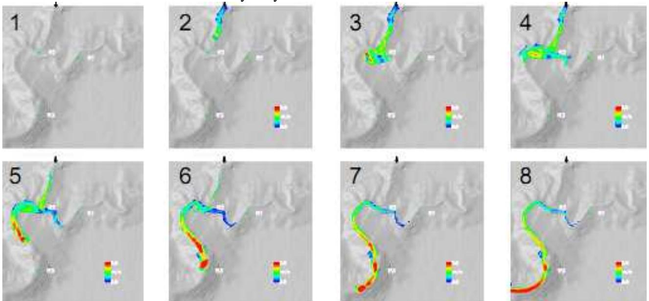
**Fig. 4.** Simulation snapshots of the December 17<sup>th</sup>, 2002, flow in the Monterey Canyon System (red = highest velocity, dark blue = lowest, near-zero velocity).
