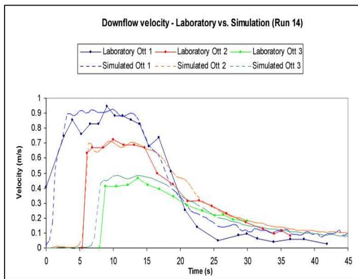
**Fig. 1.** Two-dimensional CFD simulation of a Utrecht laboratory flow: snapshots of the flow density (to the right, values in  $\text{kg/m}^3$ ) and a comparison of station-bound velocity time series (below). The flow initial sediment concentration was 25 vol.% (clay fraction, with a grain size of 0.15 mm). Arguably, the simulated velocity time series are more reliable, because the laboratory velocimeter propellers have recorded some mechanical ‘noise’ due to sediment particle entrapment.
