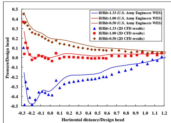
Figure 5 Comparison of crest pressure for various heads (2D model),  $H_d$  is the design head
