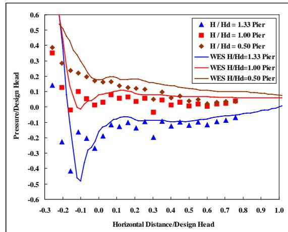
Figure 6 Comparison of crest pressure next to pier (3D model)
