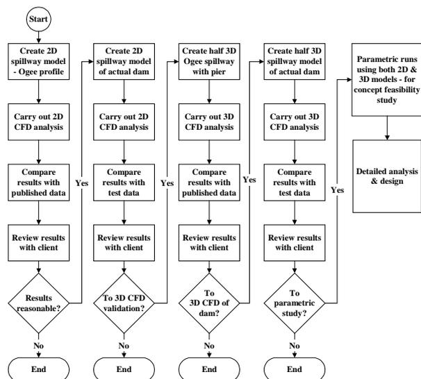
Figure 3 Flowchart showing the validation process
