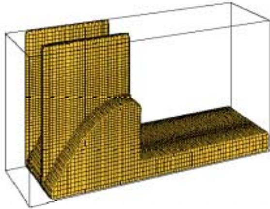
Figure 4 A view of the ogee spillway and Type 2 piers in the 3D CFD model
