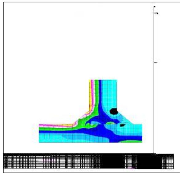
*Figure 1 Partial FE mesh of tank/foundation. Insert shows mesh and stress distribution at wall base.*
