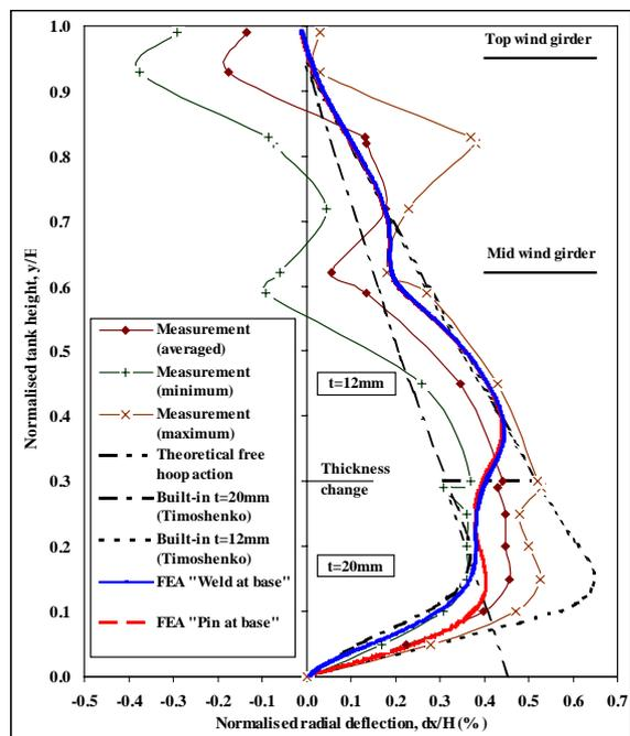
Figure 2 Wall deflection of water tank
