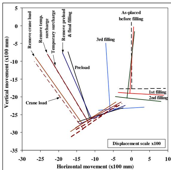
Figure 11 Wall deformations
