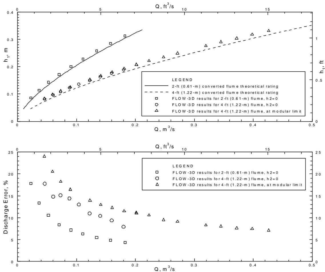
Figure 5. — Comparisons of theoretical rating curves developed using the WinFlume program and results of CFD simulations of 2 ft (0.61 m) and 4 ft (1.22 m) wide Parshall flumes converted to width-contracted long-throated flumes (upper plot). The lower plot shows the percentage errors in discharge measurement.
