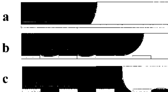
Figure 2: Flow of liquid with static contact angle 120^\circ over (a) smooth surface, (b) rough surface, and (c) liquid filled rough surface.
