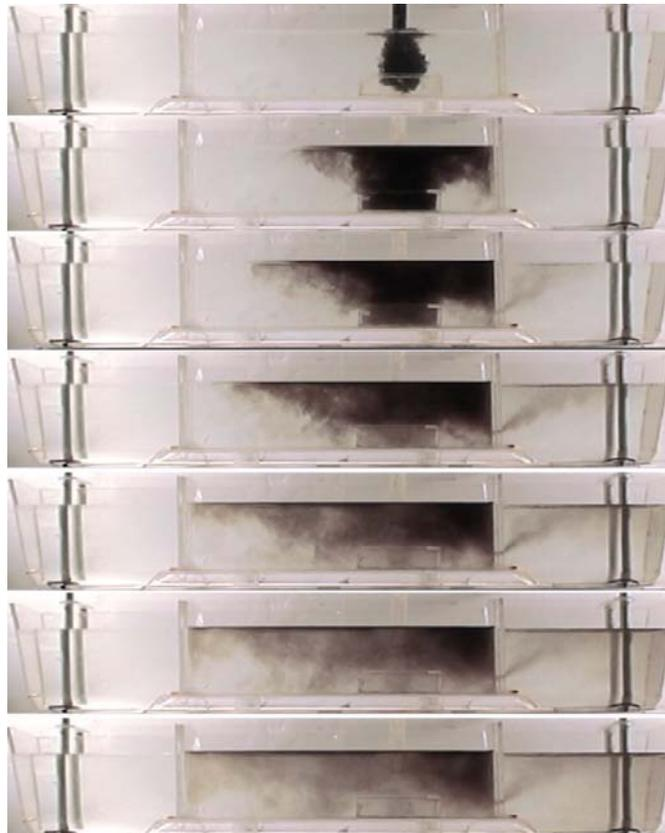
*Fig. 2. General pictures of development of fluid flow and movement of solid-liquid inclusions (black) in non-symmetric tundish with turbulence inhibitor and filter walls*
