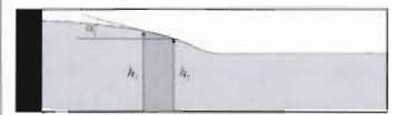
Figure 3. The illustration for calculation of the slope of the metal's free surface
