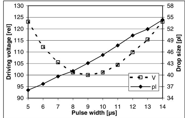
Figure 4. Measured driving voltage and drop size with constant drop speed as function of pulse width for an 8 mm channel geometry and 36  $\mu$ m nozzles.
