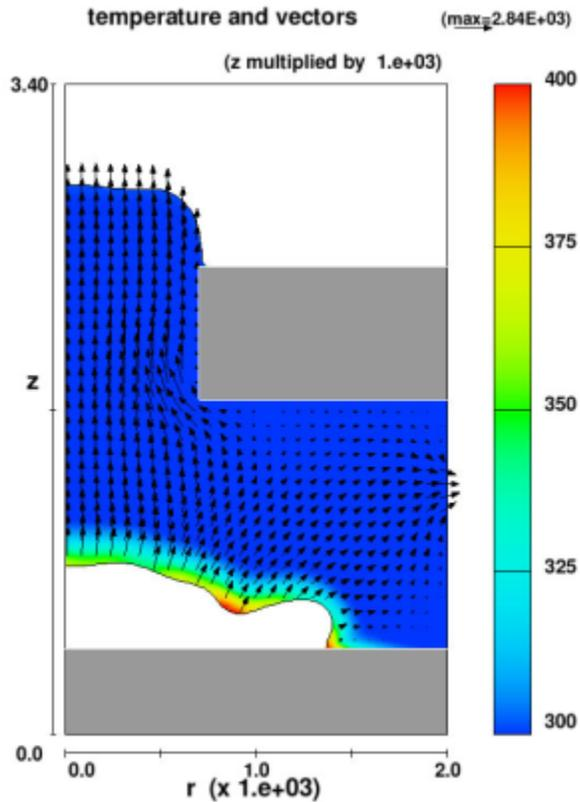
Homogeneous thermal bubble model.
