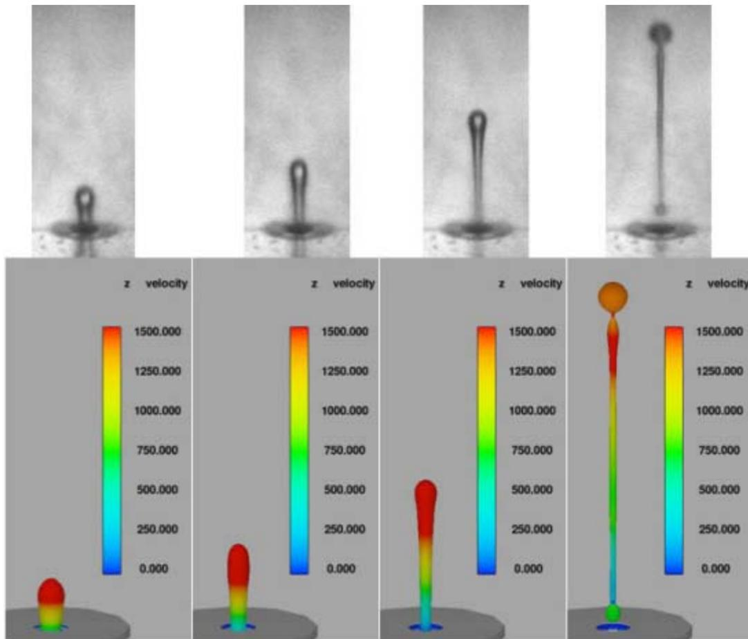
Comparison between physical experiments (top row) and simulation (bottom row) in early experimental device configuration.
