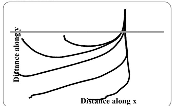
Fig. 5 Trajectories of marked points in the concrete flow during filling the mould
