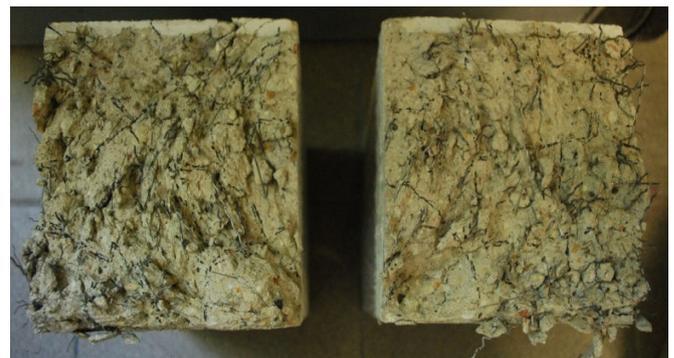
Fig. 8 Both fracture surfaces for one prism. Is possible to see many fibers oriented close to parallel to crack surface. SFRHPC with Tabix50, Dramix30, Dramix13 and Dramix6 fibers (fibers cocktail)
