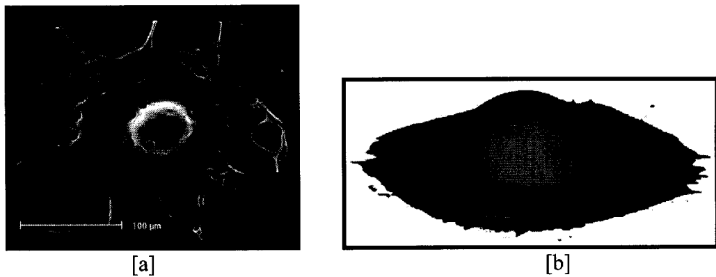
Figure 5: Static Nylon-11 splats on a room temperature flat substrate; [a] SEM micrograph, [b] 3D simulation.
