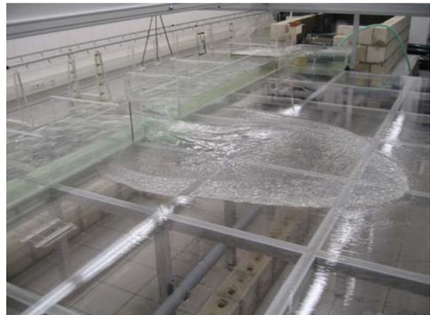
Figure 1. Sample flood wave in physical model
