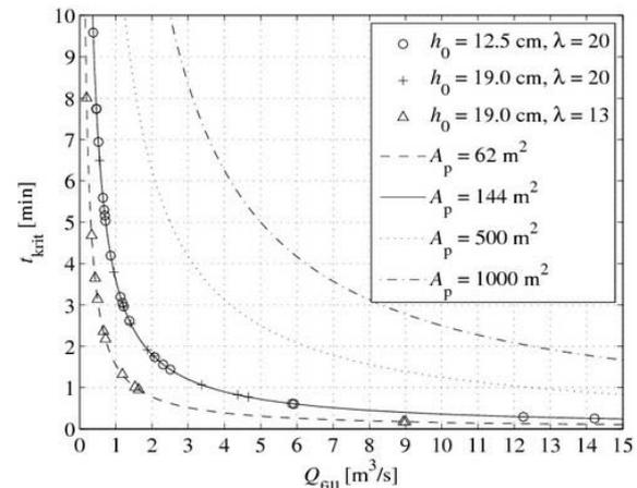
Figure 9. Critical fill times for flood-type 1
