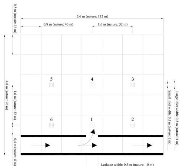
Figure 2. Technical plot of physical model
