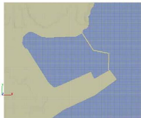
Figure 16 FEM model of port area
