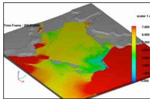
Figure 20 Water level with the flap gate
