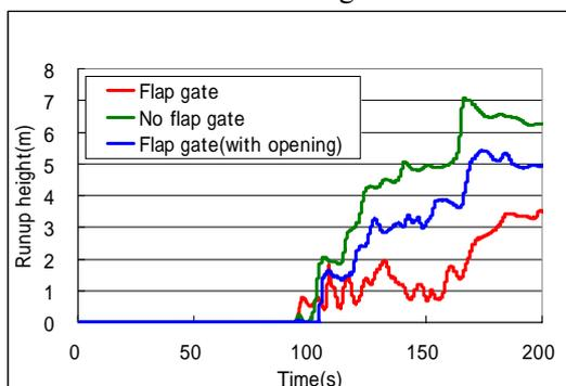
Figure 21 Run-up height at pier
