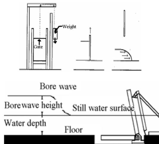
Figure 4 Generation of Tsunami (bore wave)
