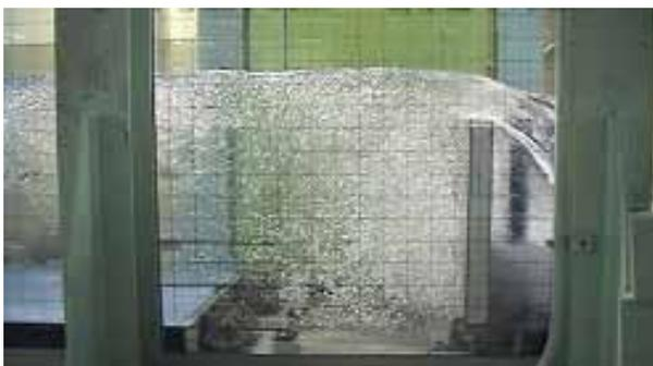
Photo 3 Overtopping at the gate (fixed type  $90^\circ$ )
