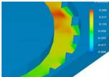
Figure 8. Flow pattern around the spur dikes in three dimensional form at numerical model
