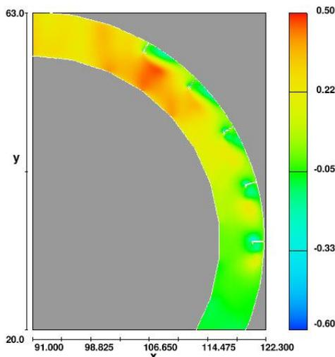
Figure 7. Distribution of the flow rate around the spur dike with a discharge of 25 liters per second
