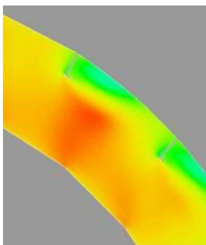
Figure 5. Speed distribution around two initial spur dikes
