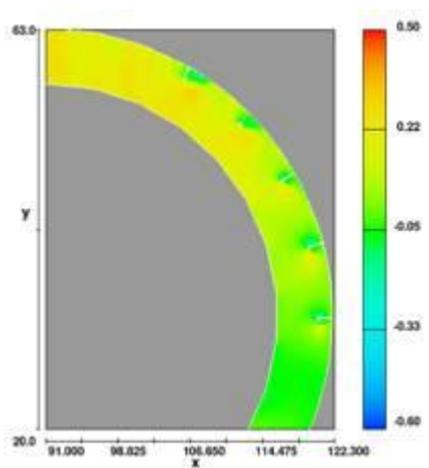
Figure 6. Distribution of the flow rate around the spur dikes with a discharge of 18 liters per second
