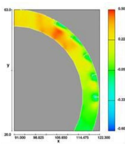
Figure 4. Distribution of speed around the spur dike series
