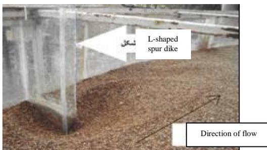
Figure 9. formation of scour and deposition around the spur dike in the original model.
