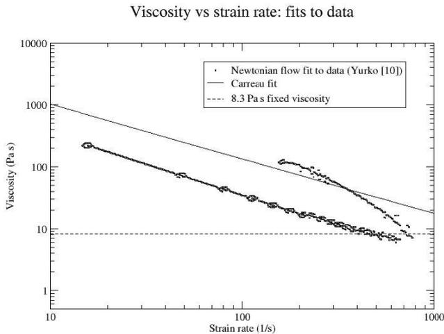
Fig. 6 : Viscosity laws for A357 at 0.49 fraction solid used to generate height vs. time data of Fig. 5
