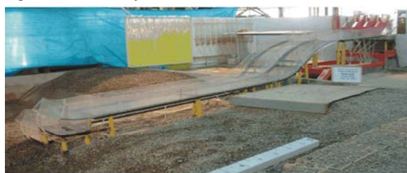
Fig. 2: Physical model of Gotvand dam's spillway-chute
