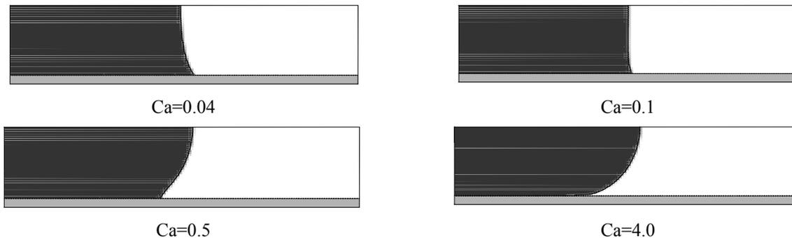
Figure 4. Dynamic contact angle computed as function of capillary number.
