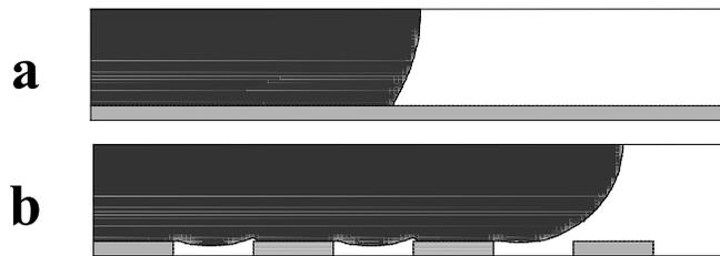
Figure 1. Flow of liquid with static contact angle 120° over (a) smooth surface and (b) a rough surface.
