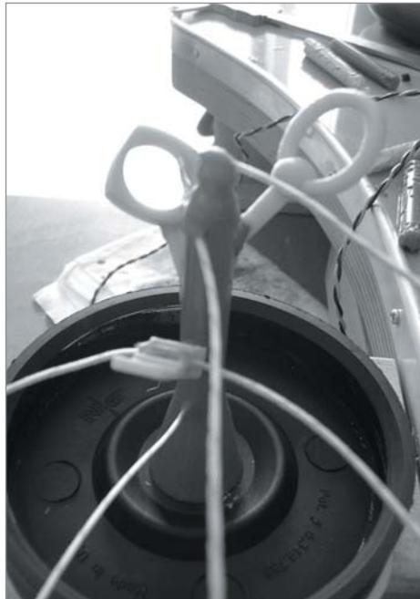
*Figure 3a Thermocouples inserted in the wax tree, side view*
