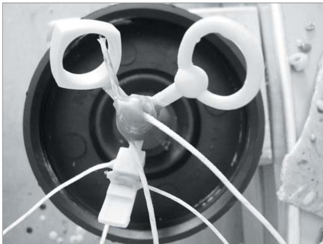
*Figure 3b Thermocouples inserted in the wax tree, top view*
