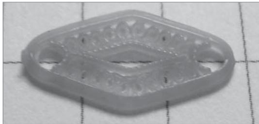
*Figure 8 Wax pattern of a “leaf” to be modelled and studied*
