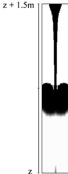
Fig. 5. Sheared and resting zones in a wall formwork. SCC is cast from the top of the formwork at a casting rate of 5 m/h. In the black zone, the shear rate is greater than  $0.1 \text{ s}^{-1}$  (from [12]).
