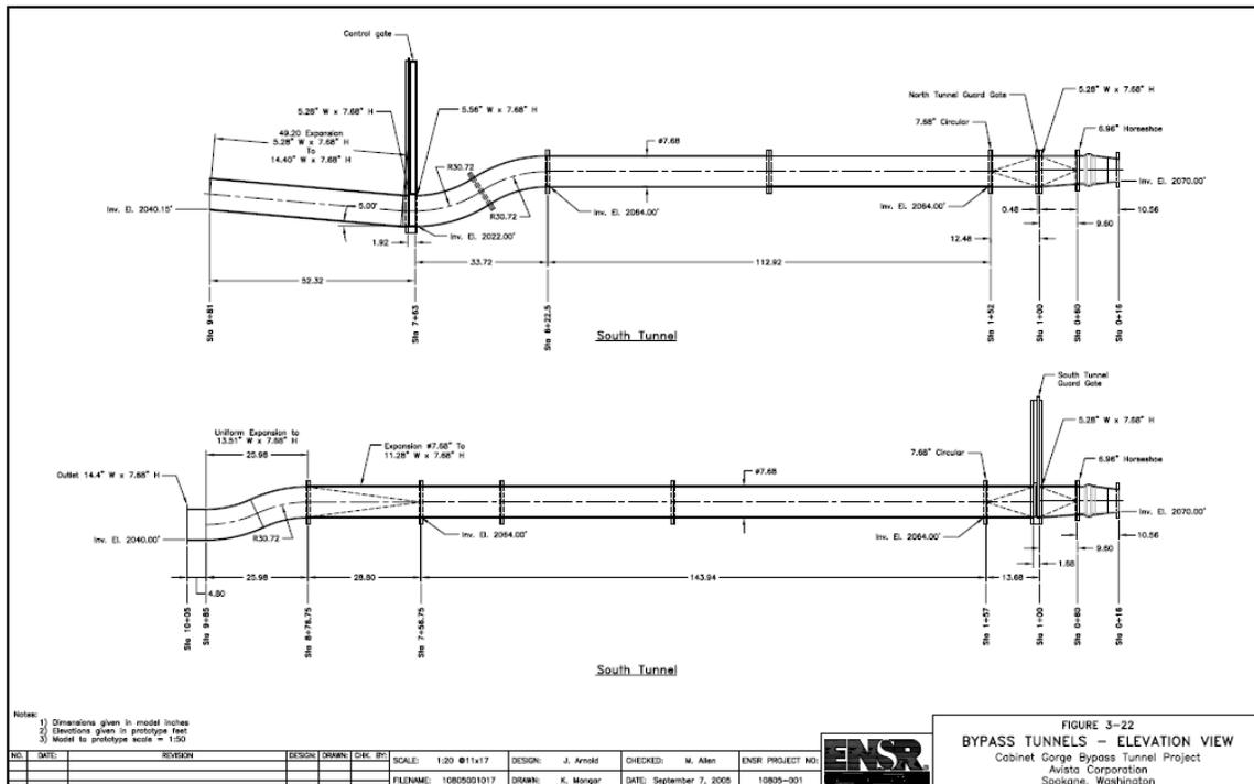
Figure 2.3: Elevation view of the tunnels
