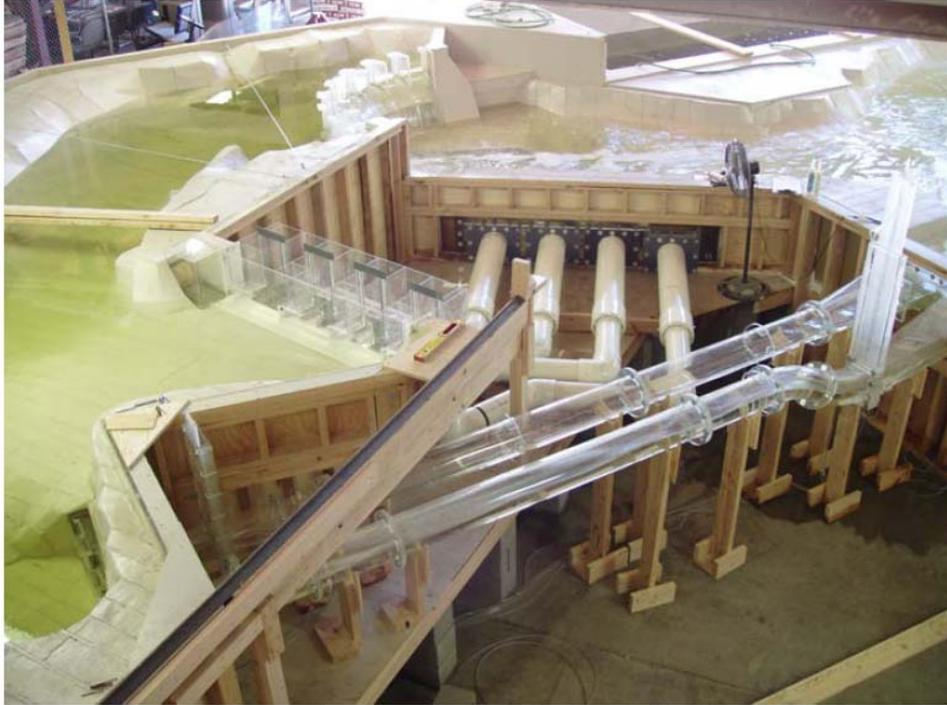
Figure 2.2: Physical model overview with bypass tunnels in foreground
