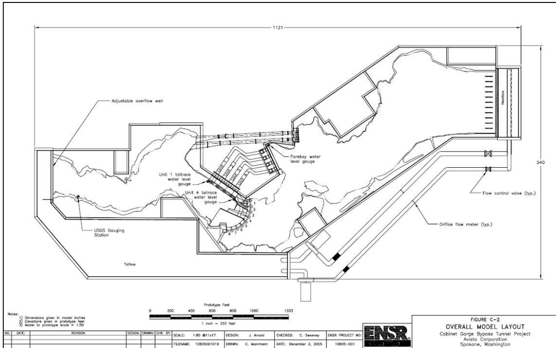
Figure 2.1: Overall layout of Cabinet Gorge physical model
