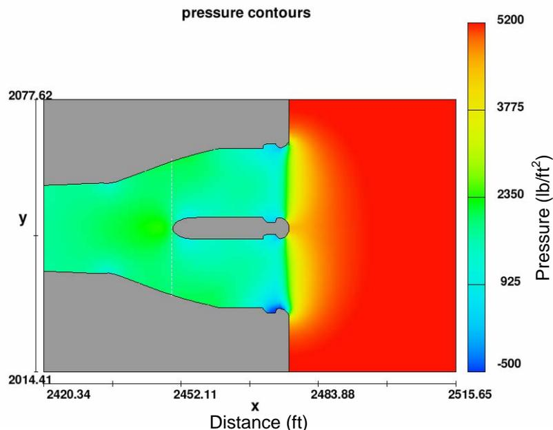
Figure 3.2: Pressure distribution for tunnel discharge of 38,000 cfs
