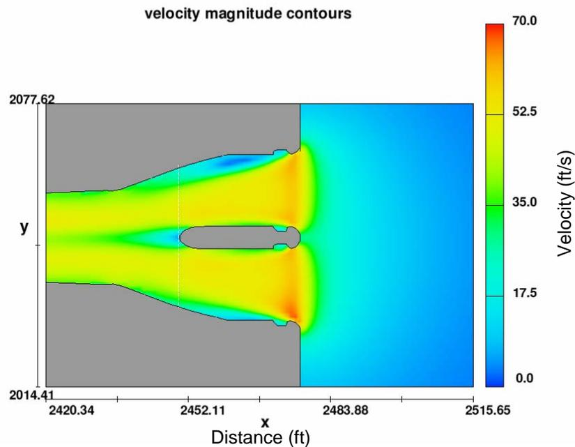
Figure 3.3: Velocity distribution for tunnel discharge of 38,000 cfs
