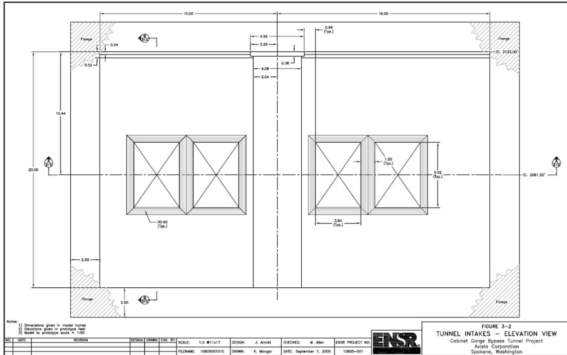
Figure 2.4: Frontal elevation view of tunnel entrances
