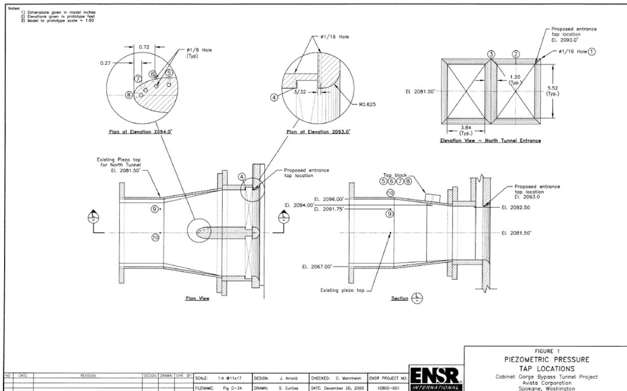
Figure 2.5. Pressure tap locations in North Tunnel inlet
