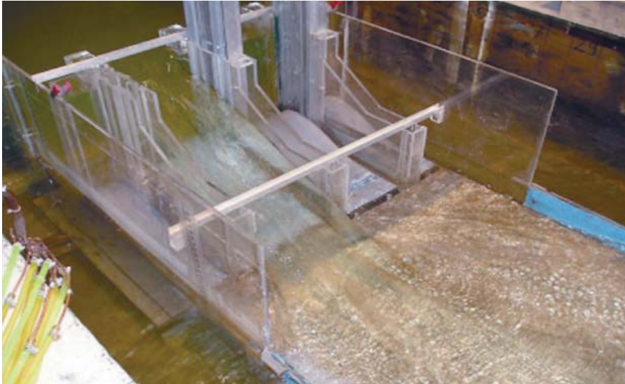
This partial model of the spillway for the proposed 675-MW Keeyask station was developed to confirm rating curves for full and partial gate openings for both diversion and final rollway conditions, as well as to verify pressures and gate behavior.
