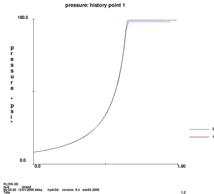
**Figure 5:** Pressure curves from the "All Closed" for 1-compressible and 2-adiabatic simulations.
