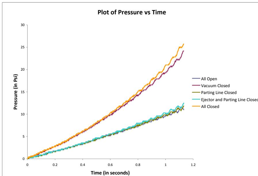
**Figure 3:** Experimental results of pressure (in Psi) plotted against time (in sec) for the dry runs.
