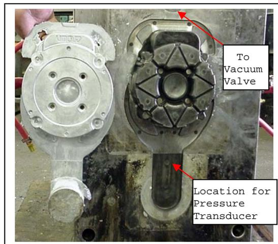
**Figure 2:** The cast part (end head of motor) and the die.
