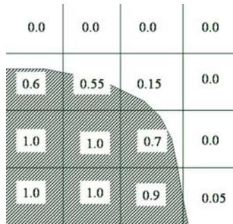
**Figure 1:** Typical values of the VOF function near a moving metal front.
