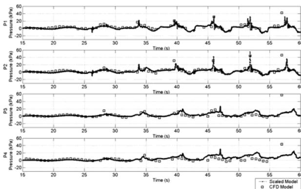
Figure 7 Hydrodynamic pressure under the wharf from CFD and Scale test
