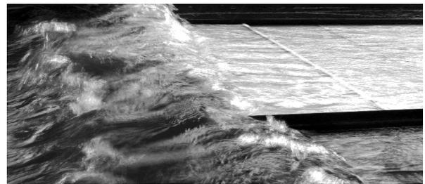
Figure 6 Scaled structure overtopping (H=2.9m, T=6s)
