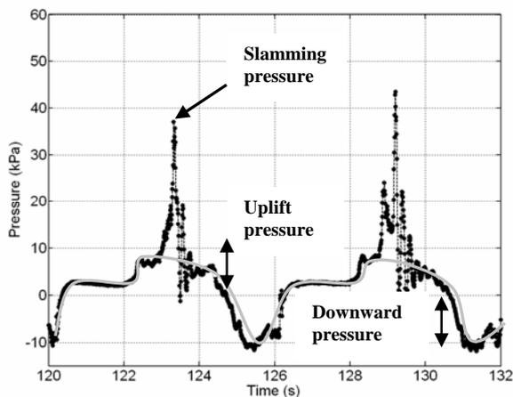
Figure 2 Definition of wave pressure parameters, from a pressure transducer record
