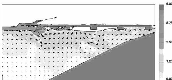
Figure 5 CFD model wave overtopping (H=2.9m, T=6s), shading indicates fluid velocity, m/s
