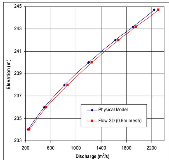
Figure 2. Wuskwatim discharge rating curves.
