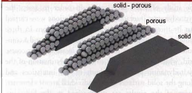
Fig.2a: Submerged Breakwaters
