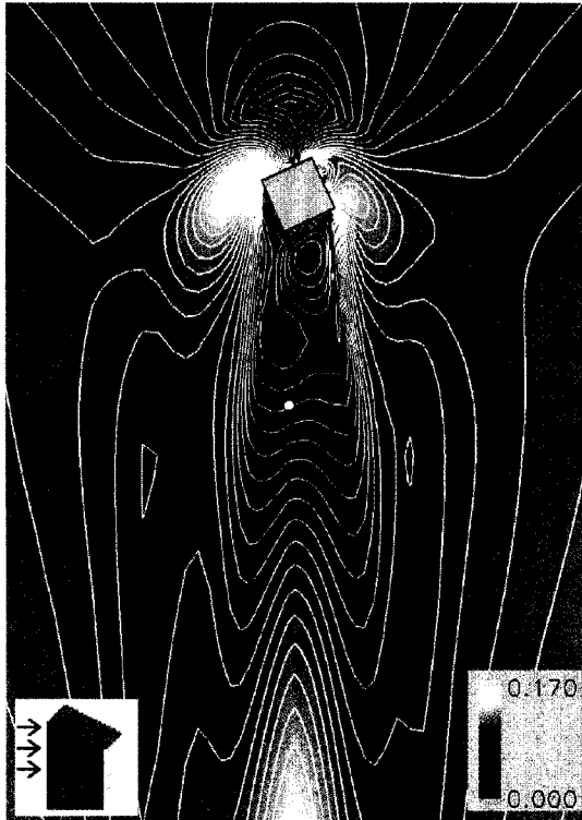
3. c) case c) calculated shear stress around a single pitch roofed building with the highest wall towards the wind. The downwind reattachment point is indicated with a white dot, colour scale in \text{N/m}^2 , contour line spacing is 7.7 \cdot 10^{-3} \text{ N/m}^2 .
