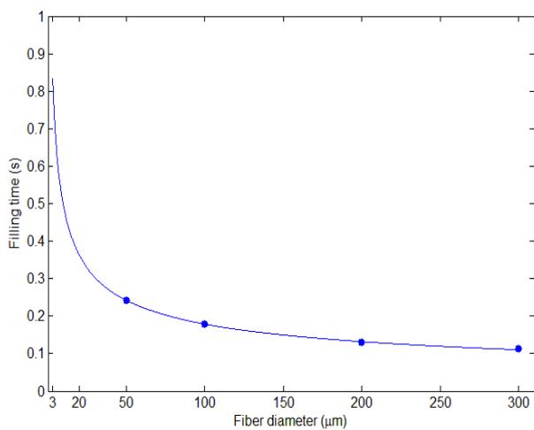
Fig. 10. Relationship between fiber diameter and filling time
