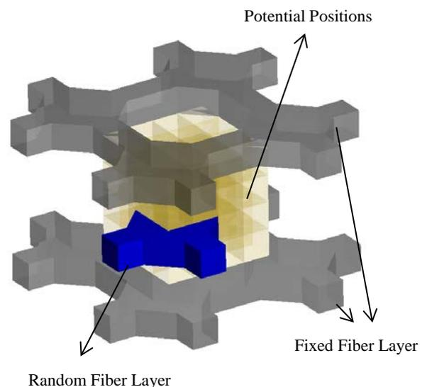
Fig. 4. The placement of the fiber layers
