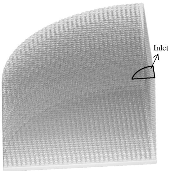
Fig. 6. Computational domain in the CFD model
