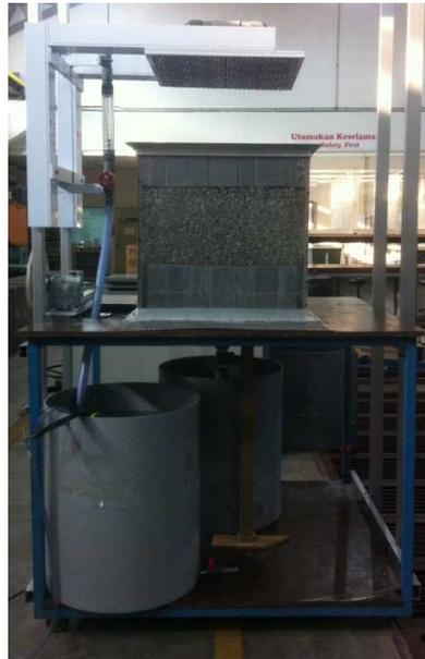
**Figure 1:** Physical model of the permeable pavement in laboratory
