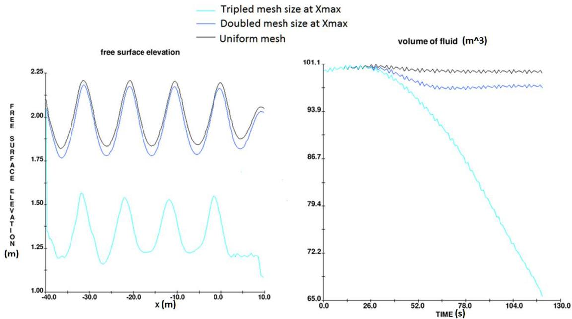
Figure 13. Wave profiles at 120 s and time variation of water volume for different mesh size distributions in the horizontal direction in the sponge layer
