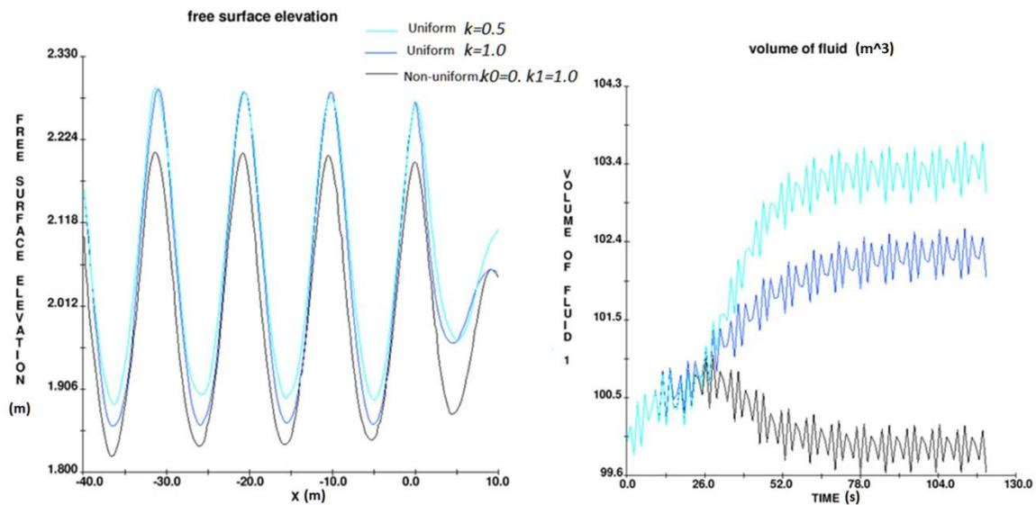
Figure 12. The wave shape at 120 s and time variation of the water volume for different damping coefficient distributions.
