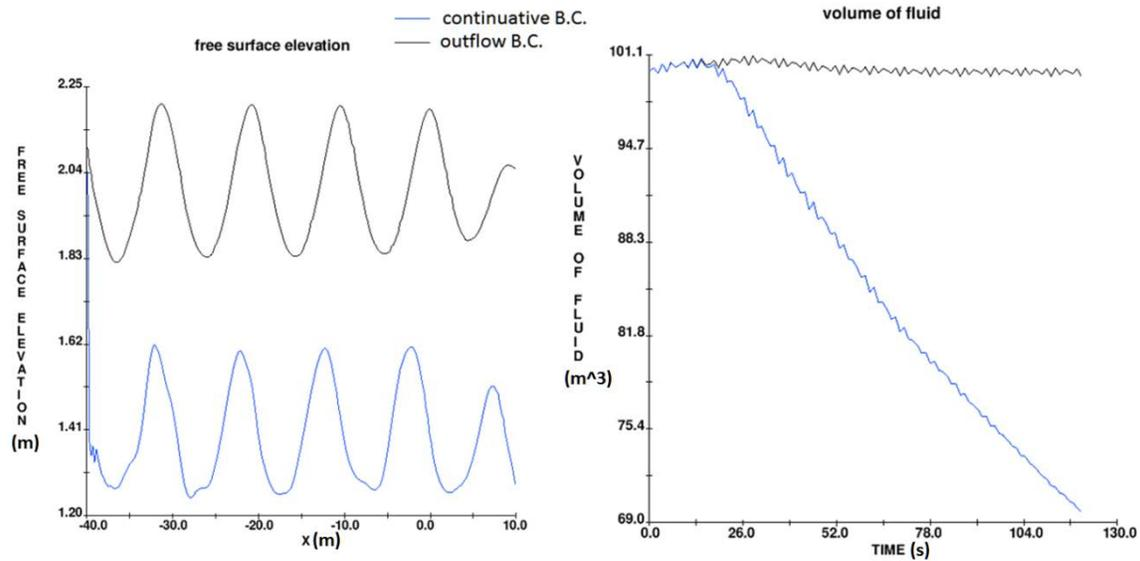
Figure 14. Wave profiles at 120 s and time variation of the water volume for different boundary conditions at the open boundary.
