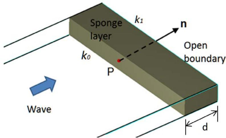
Figure 3. A sponge layer and the artificial damping coefficient.
