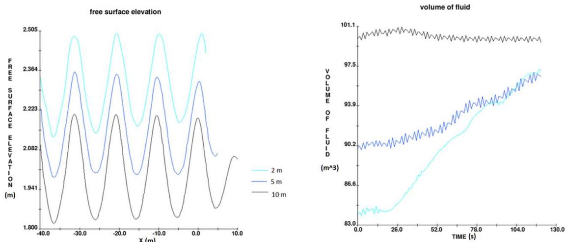
Figure 11. Wave profiles at 120s and variation of water volume with time for different sponge layer lengths.
