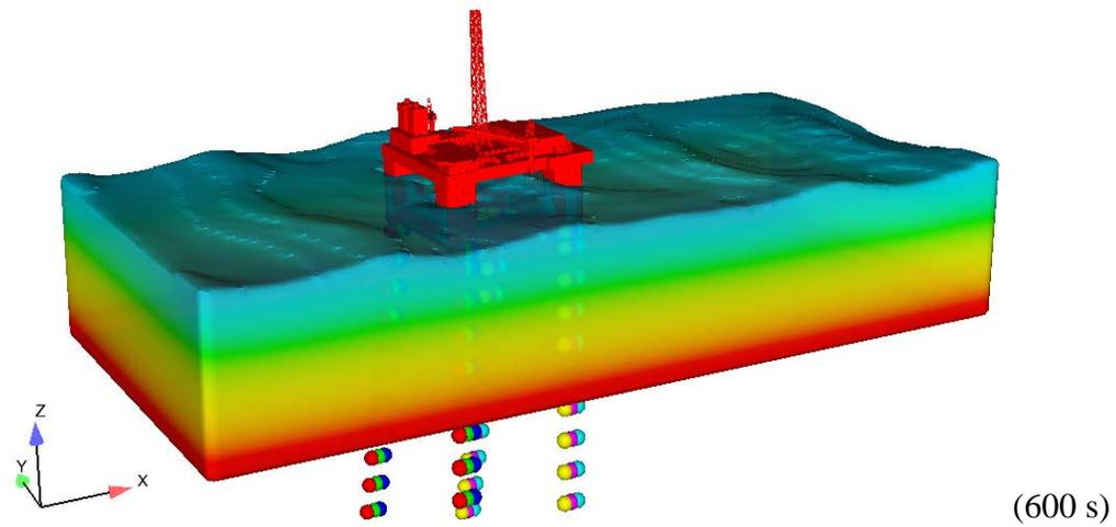
Figure 7. A wave passing around a moored platform, when a radiation boundary condition is used but not the sponge layer. Color denotes pressure.
