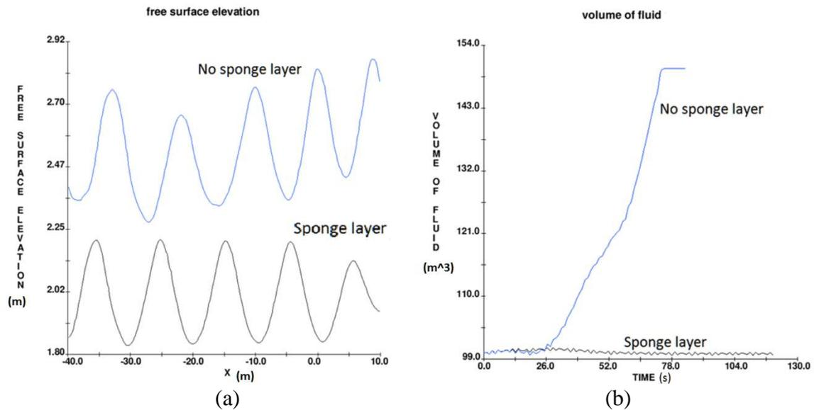
Figure 5. Comparison of simulation results with and without a sponge layer.
