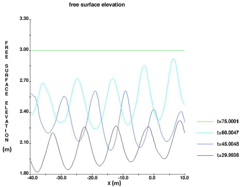
**Figure 1.** The wave profile versus time using the radiation boundary condition.
