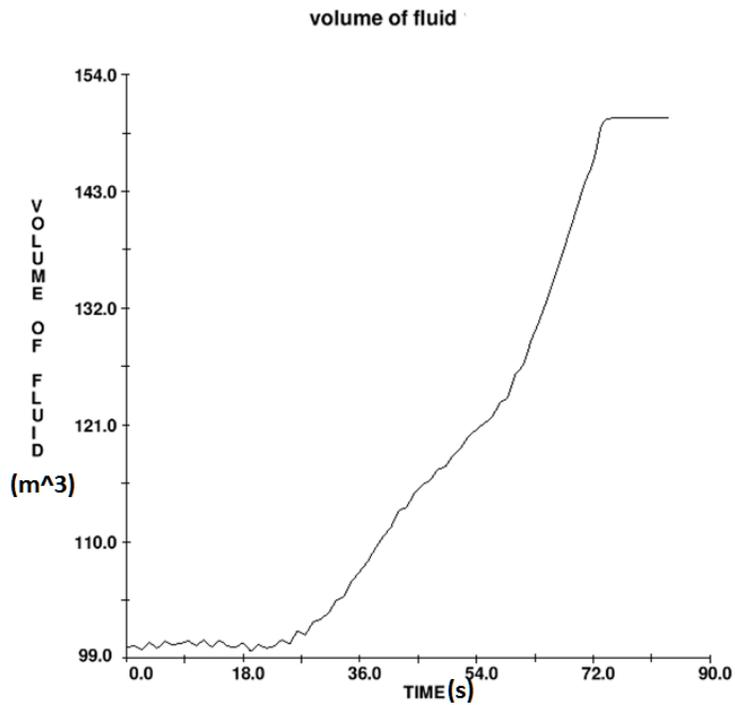
**Figure 2.** The total water volume versus time using the radiation boundary condition.
