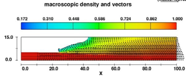
Figure 3b. Hydraulic jump in the conduit.
