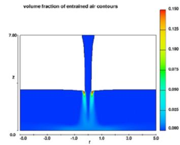
Fig.1c. Air entrained with 2% turbulence in the jet.
