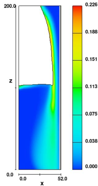
Figure 2b. Volume fraction of air entrainment in the drop shaft.
