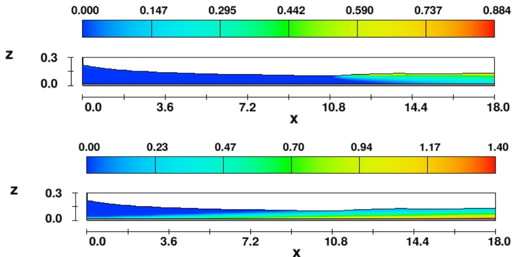
Figure 4. Entrained volume fraction of air (top) and turbulent kinetic energy (bottom).
