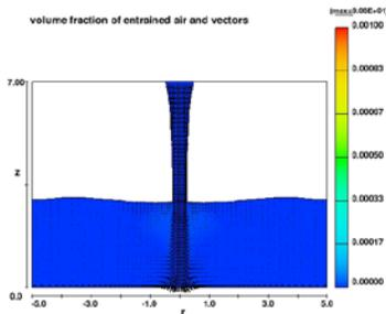
Fig.1a. Computed air entrained without turbulence.
