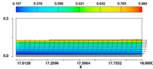
Figure 5. Volume fraction of air and velocity vectors in the last 1 m of the model spillway. Very slight changes are seen with respect to distance along the spillway.
