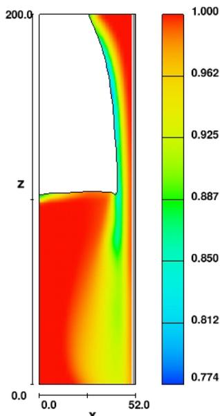
Figure 2a. Variable density in drop shaft flow indicates air entrainment.
