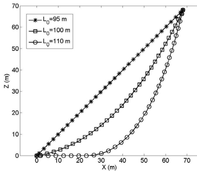
**Figure 5.** Equilibrium shapes of cables of different length using *FLOW-3D*.
