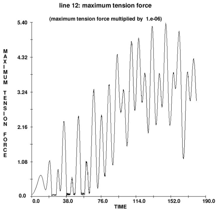
Figure 10. Maximum tension (in N) versus time (in s) for the mooring lines at the front (a) and back (b) of the platform.
