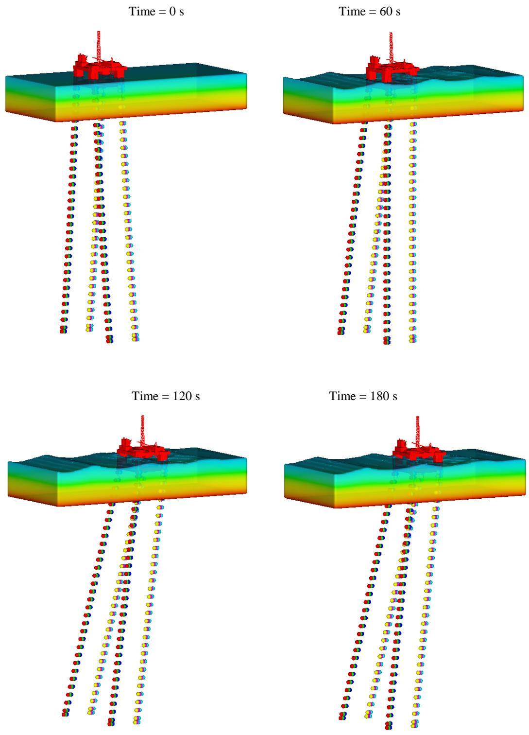
Figure 7. The platform and the wave motion at four different times. The mooring lines are shown as strings of dots. Color represents pressure in the water.
