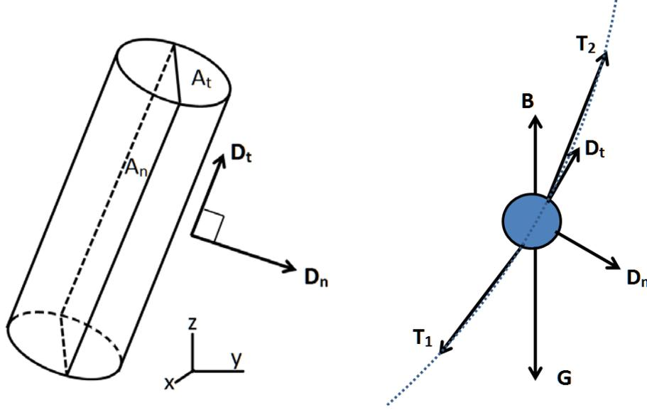
**Figure 2.** Forces applied to a mooring line segment at its mass point.
