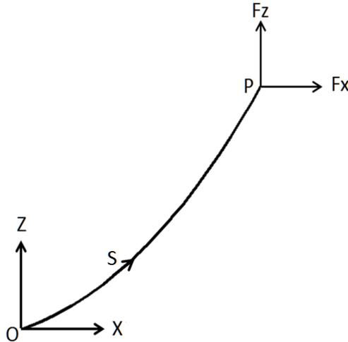
**Figure 3.** Coordinate system and forces for the elastic catenary.
