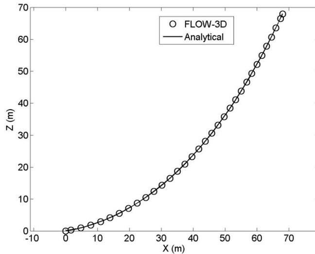
**Figure 4.** *FLOW-3D* result and analytical solution for an elastic catenary.
