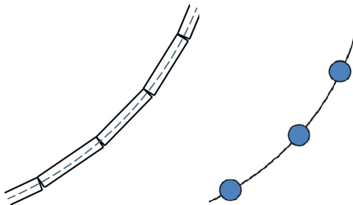
**Figure 1.** Discrete segments of a mooring line and the mass point representation of the segments.
