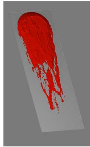
Figure 14c. Flow after 5s when the initial solid fraction has been set at its maximum value. Plotted surface is fluid fraction of 0.2.
