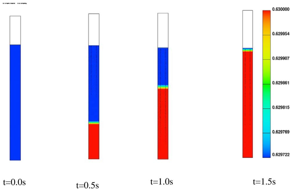
Figure 1. Color is solid fraction of mixture: 0.55 initially and 0.63, the maximum close packing after settling. Gas escape at top can be seen to reduce the height of the column.
