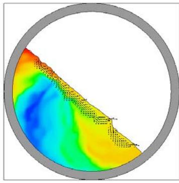
Figure 5b. Simulation of rotating mixer: after 2 revolutions.
