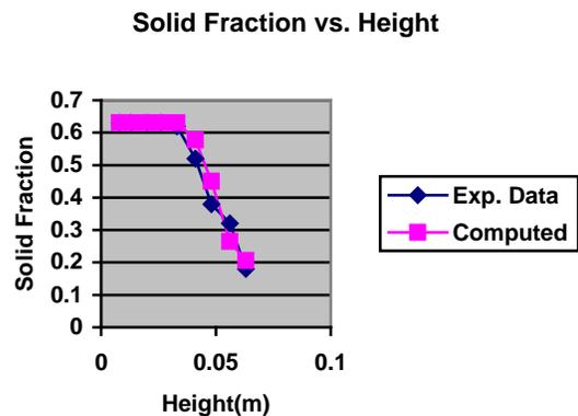
Figure 10b. Comparison of experimental Run #85 from [7] and computed data for solid fraction as a function of height above channel floor.
