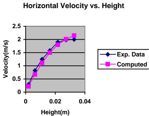
Figure 11a. Comparison of experimental Run #46 from [7] and computed data for horizontal velocity as function of height above channel floor.
