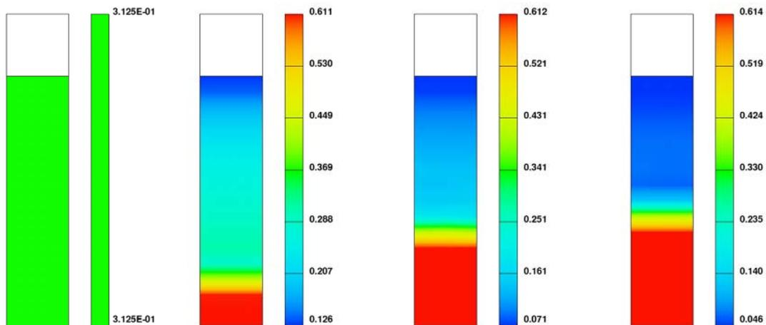
Figure 7a. Color indicates solid fraction in granular mixture. Initial solid fraction is 0.3125. Subsequent frames are at times 1s, 5s and 20s. At late time there is a region of nearly pure water (solid fraction less than 5%) separating air from the packed solid at the bottom of the column. Also note that there is no net volume change in the water/solid mixture as the solid settles; compare with Fig.1 for an air/solid mixture.
