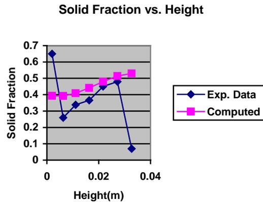
Figure 11b. Comparison of experimental Run #46 from [7] and computed data for solid fraction as function of height above channel floor.
