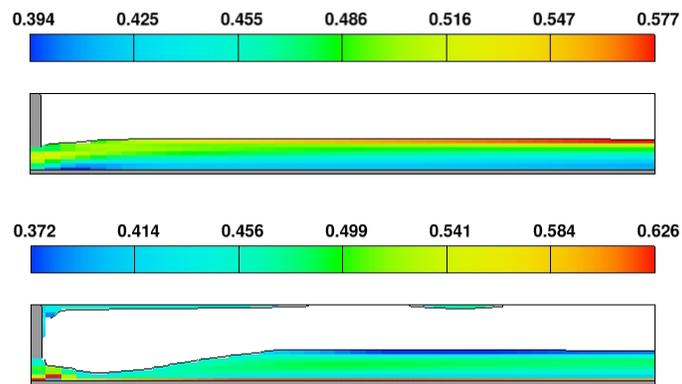
Figure 12. Comparison of flow in first 0.8m of flume for Run #46 from [7] with dispersive pressure (top) at steady conditions and after another 0.2s (bottom) without a dispersive pressure. Color indicates solid fraction.
