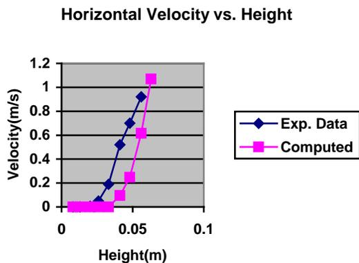
Figure 10a. Comparison of experimental Run #85 from [7] and computed data for horizontal velocity as a function of height above channel floor.
