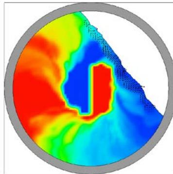
Figure 4b. Simulation of rotating mixer: after 2 revolutions.
