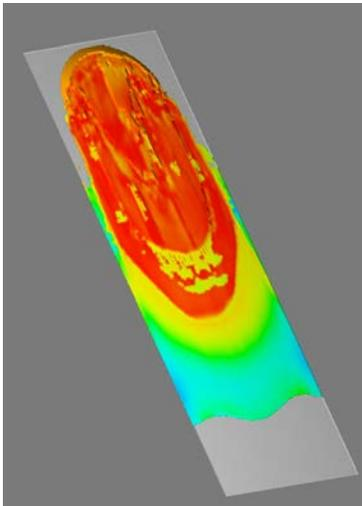
Figure 14b. Flow after 5s. Color is solid fraction and shows how settling sand has allowed the mixture to flow further down the slide.
