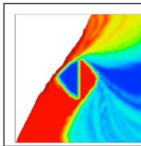
Figure 6b. Simulation of rotating rectangular mixer after 1.25 revolutions.
