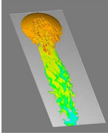
Figure 13b. Flow of sand after 5s. Color is solid fraction. The plotted surface is fluid fraction 0.2.
