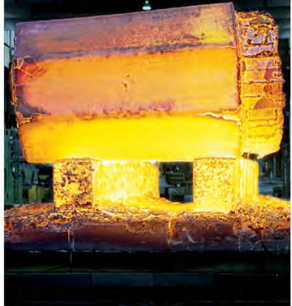
Thermodur® Hot Work Die Steels are engineered for maximum toughness and thermal fatigue resistance under extreme conditions.
