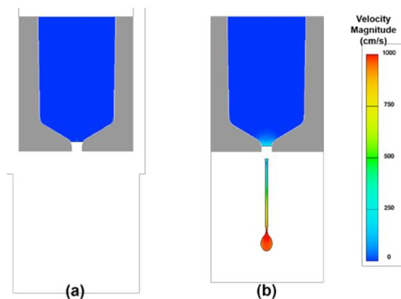
**Figure 3.** CFD analysis of droplet generation showing fluid velocity magnitude (cm/s): (a) fluid is at rest in the ejection chamber before the onset of the ejection pressure, (b) droplet ejection due to the applied pressure pulse of Fig. 2b.
