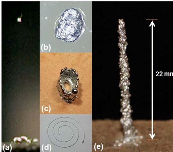
**Figure 4.** Droplet generation and droplet-media interactions: (a) jetted aluminum droplet in flight, (b) aluminum droplet solidified on a plastic substrate, (c) solidified printed ring structure, (d) spiral pattern of printed droplets after solidification, (e) printed pillar of coalesced aluminum droplets.
