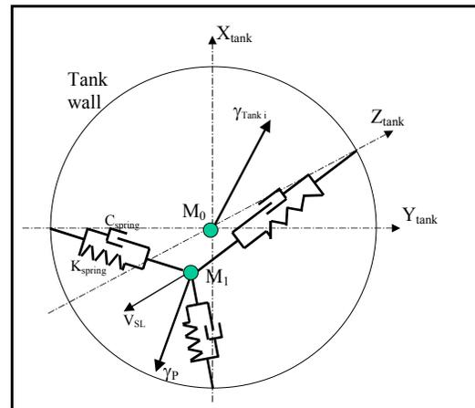
Figure 7 : Sloshing mechanical model for the docking phase
